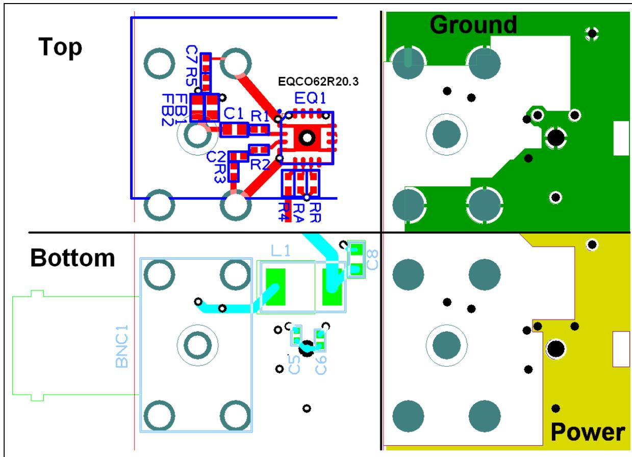
In this layout, the size of the PCB area needed for the chip is minimized. Approximately two times the BNC footprint area is required for the full bidirectional system: including the necessary elements for the power transport.
