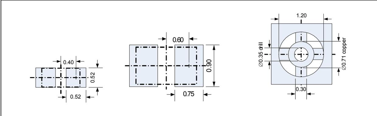
FIGURE E-2: DIN1.0/2.3 AND L1 INDUCTOR 1812 FOOTPRINTS
