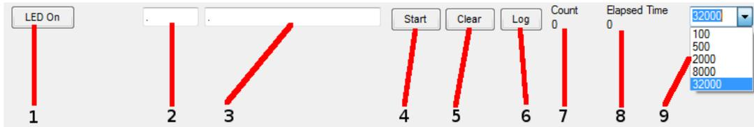
1. Toggles LED on the controller board.
