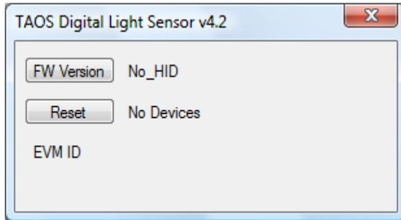
If “No Devices” appears, verify that the daughterboard is connected to the motherboard properly. If “No\_HID” appears, verify the USB cable is connected. A green LED on the motherboard indicates that the USB cable is connected and providing power to the system.
