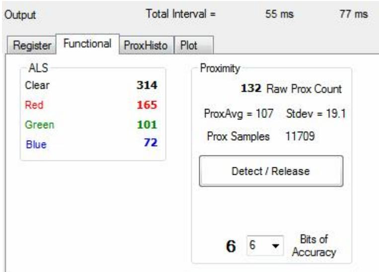
The Prox indication shows the current reading (Raw number) and the rolling average. The average is computed over the number of samples specified on the INPUT/Functional tab.
