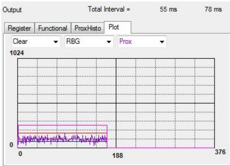
The graph shows all outputs for a static system. The X-axis plots 376 points then rolls over back to 1 on the graph. The Y-axis is set to range 0 to 1024; this range cannot be adjusted. However Multipliers (selected from the list boxes) may be used to scale the display accordingly.
