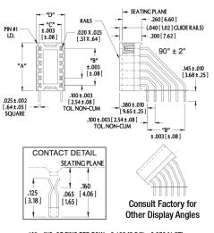
"A"= (NO, OF PINS PER BOW x 0.100 [2.54]) +0.050 [1.27] "B"= (NO. OF PINS PER ROW -1) x 0.100 [2.54]
