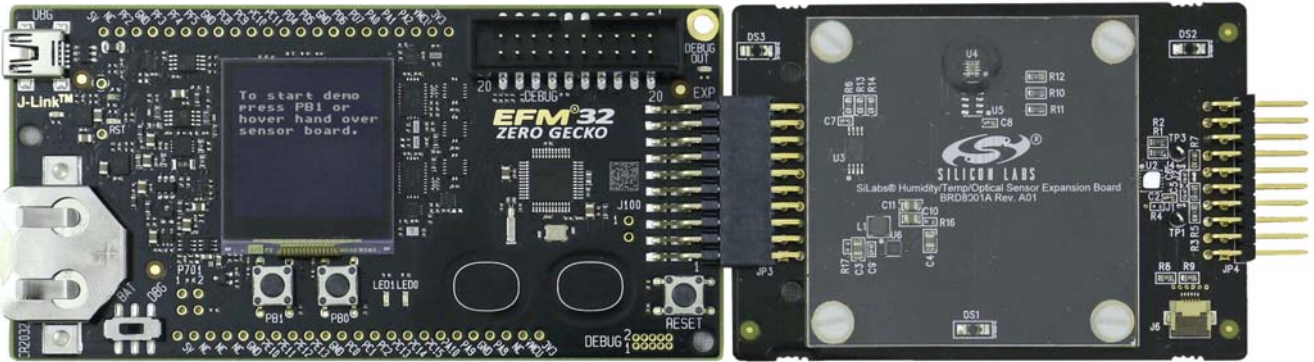
Figure 8. Sensor-EXP-EVB Connected to Zero Gecko STK
