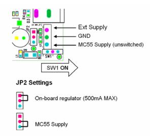
SW1 (slide switch) provides the power on / off for the module but does not isolate the power from other components of the development board.
