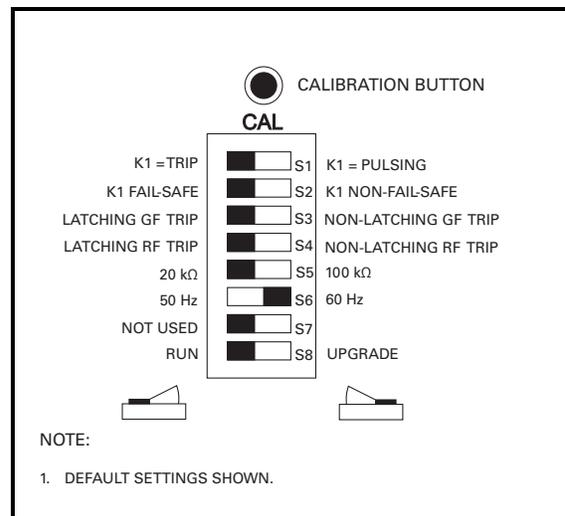
FIGURE 1. Configuration Switches.
