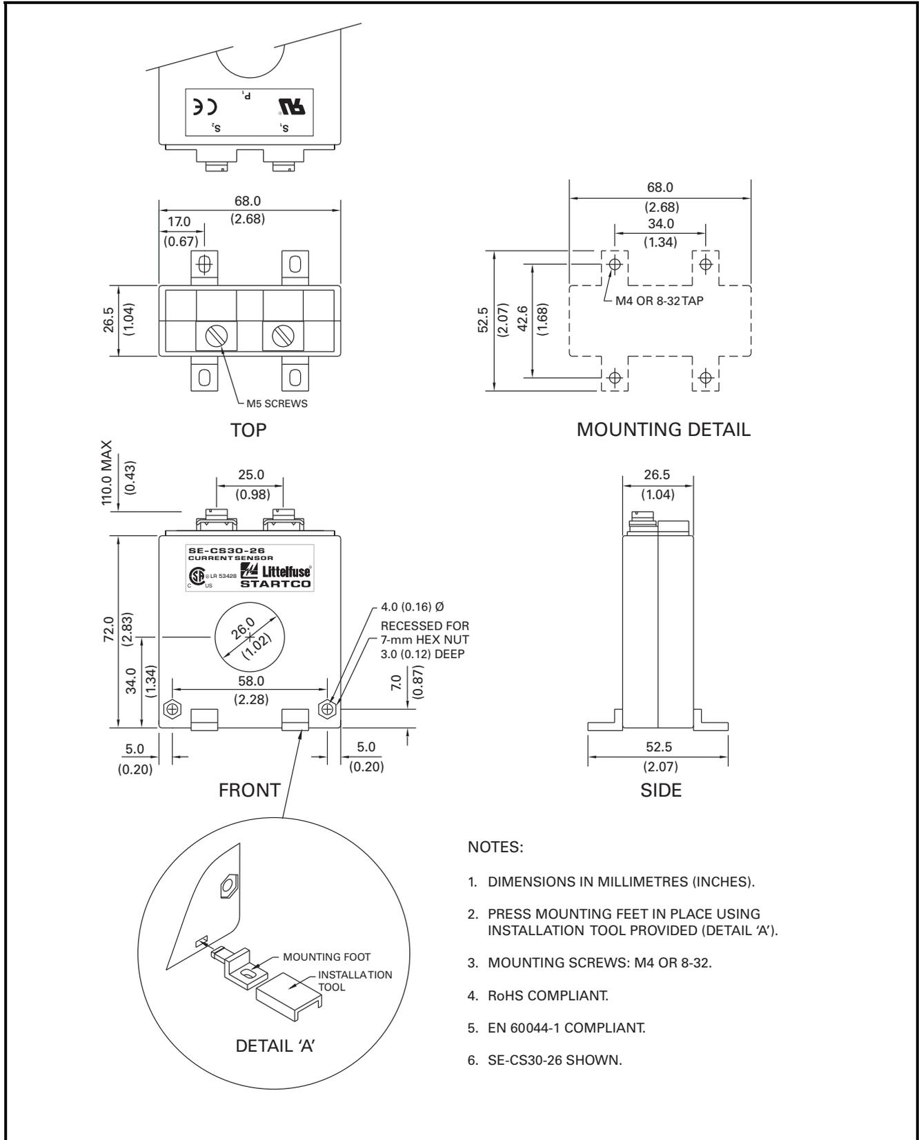
FIGURE 18. EFCT-26 and SE-CS30-26 Ground-Fault Current Sensors.
