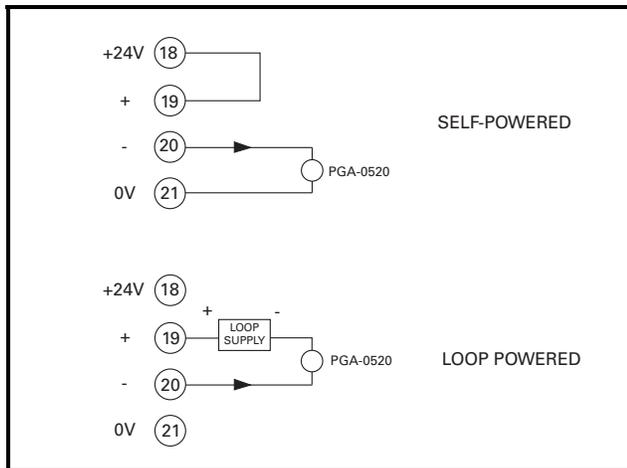
FIGURE 2. Analog-Output Connections.
