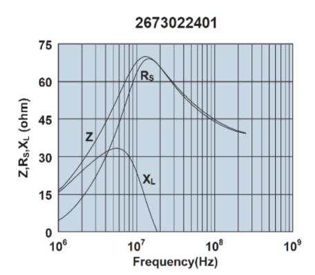
Impedance, reactance, and resistance vs. frequency.
