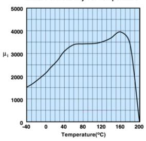
Measured on a 17/10/6mm toroid at 10kHz.
