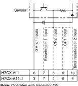
Note: Operates with transistor ON
