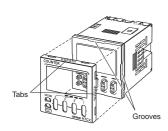
The Front Panel is attached to the Counter/Tachometer with tabs in four locations. To remove the Front Panel, open the tabs and pull the Front Panel forward. To attach the Front Panel, press it onto the Counter/Tachometer so that all four tabs lodge into the grooves on the body of the Counter/Tachometer.
