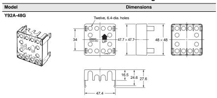
Note: The Terminal Cover can be used with a Back-mounting Socket (P3GA-11) to create a finger-safe construction.
