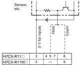
Note: Operate when the transistor turns ON
