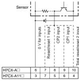
Note: Operates with transistor ON.
