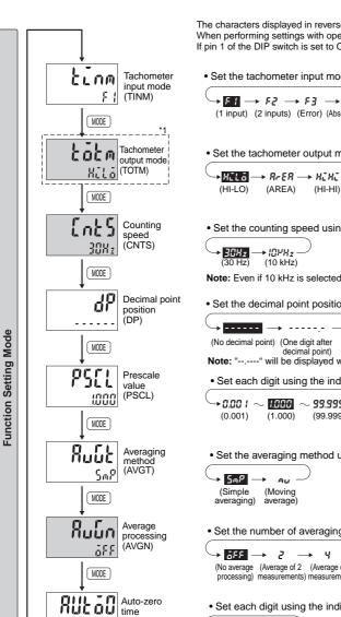
The characters displayed in reverse video are the default settings. When performing settings with operation keys only, set pin1 of the DIP switch to OFF (factory setting). If pin 1 of the DIP switch is set to ON, the setting items indicated by will not be displayed.
