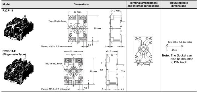
Note: Round crimp terminals cannot be used on Finger-safe Sockets. Use forked crimp terminals.
