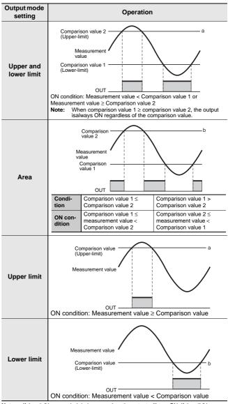
Note: If time "a" is exceeded during operation, the output will turn ON. If time "b" is exceeded during operation, the output will turn OFF. (If average processing is enabled, the output operation will be performed when the time is exceeded once.)
