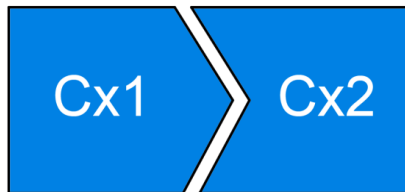
Figure 6.1 : Self Capacitance Swipe Switch Sample Electrodes.
