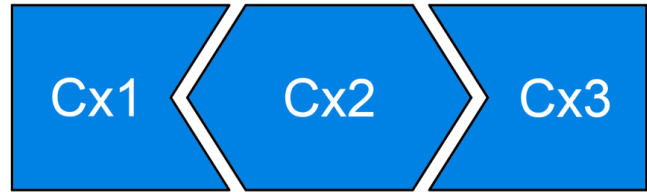
Figure 6.1 : Self Capacitance Swipe Switch Sample Electrodes.
