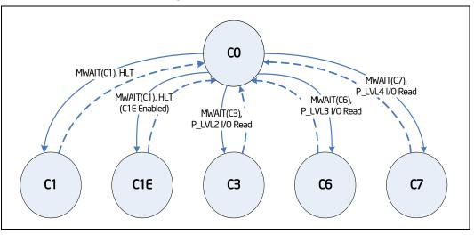
While individual threads can request low power C-states, power saving actions only take place once the core C-state is resolved. Core C-states are automatically resolved by the processor. For thread and core C-states, a transition to and from CO is required before entering any other C-state.
