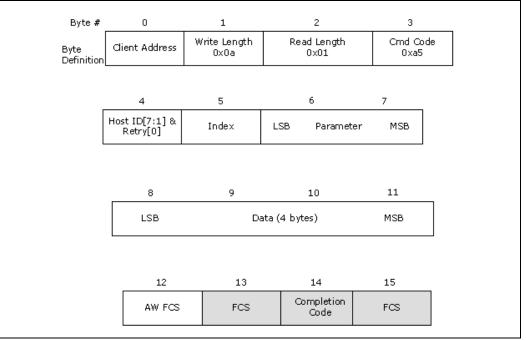
*Note:* The 2-byte parameter field and 4-byte write data field defined in Figure 2-11 are sent in standard PECI ordering with LSB first and MSB last.
