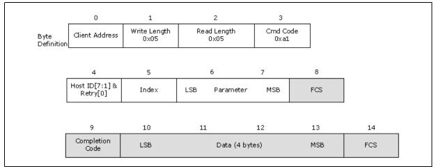
Note: The 2-byte parameter field and 4-byte read data field defined in Figure 2-10 are sent in standard PECI ordering with LSB first and MSB last.
