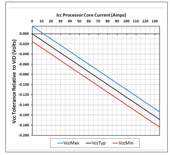
Figure 7-3. V<sub>CC</sub> Static and Transient Tolerance Loadlines
