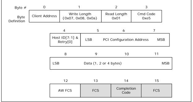
Note: The 3-byte PCI configuration address and write data field defined in Figure 2-48 are sent in standard PECI ordering with LSB first and MSB last.
