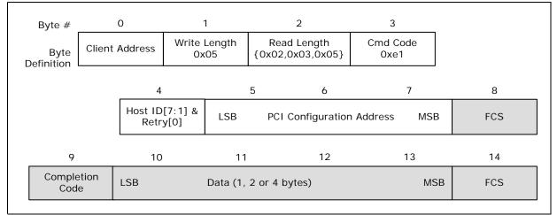
*Note:* The 3-byte PCI configuration address and read data field defined in Figure 2-47 are sent in standard PECI ordering with LSB first and MSB last.
