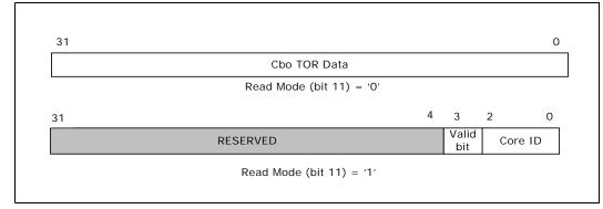
*Note:* Reads to caching agents that are not enabled will return all zeroes. Refer to the debug handbook for details on methods to interpret the crash dump results using the Cbo TOR data shown in Figure 2-40.
