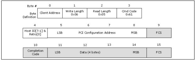
*Note:* The 4-byte PCI configuration address and read data field defined in Figure 2-45 are sent in standard PECI ordering with LSB first and MSB last.
