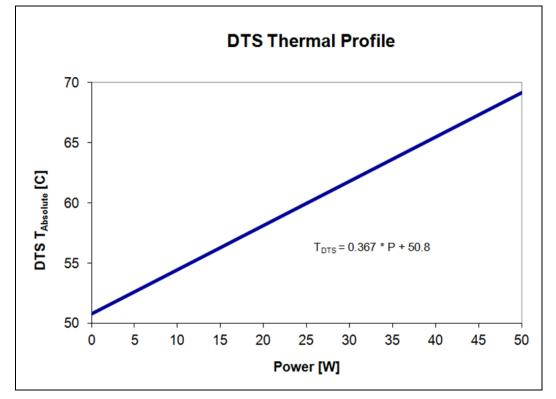
Table 5-13. Server SKU Platform (8-Core 50W) T<sub>CASE</sub> and DTS Based Thermal Profiles
