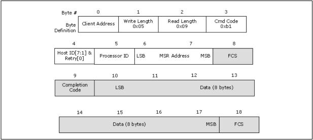
Note: The 2-byte MSR Address field and read data field defined in Figure 2-43 are sent in standard PECI ordering with LSB first and MSB last.
