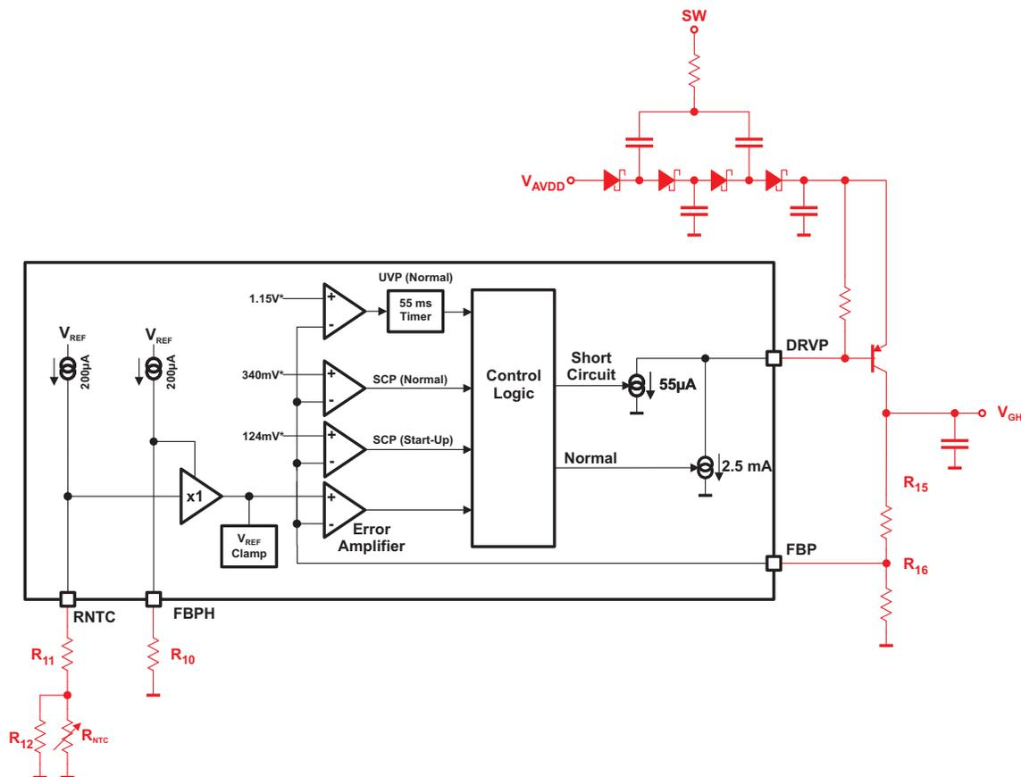
Figure 30. Positive Charge Pump Internal Block Diagram
