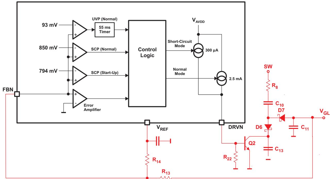
Figure 33. Negative Charge Pump Internal Block Diagram
