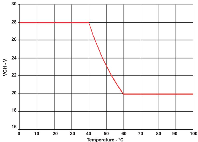
Figure 32. Temperature Compensated V<sub>GH</sub>
