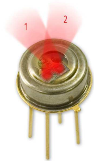
Figure 30: Identification of zone 1&2 relative to alignment tab
