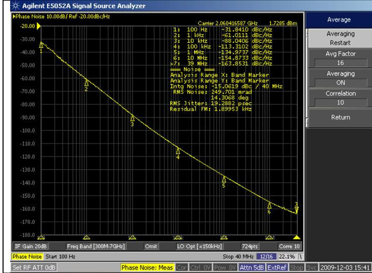
To measure the VCO phase noise, a simple technique is to lock the PLL to the desired frequency and set the charge pump state to "Tri-State", by clicking this on the PLL tab on Codeloader. If the phase noise analyzer can track the signal, a reasonable measurement can be made. To ensure that this measurement is of the VCO noise, omit the the spurs and disconnect the microwire programming cable.
