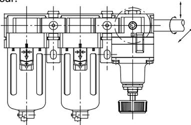
3. Since excessive moment loads and the propagation of vibrations, etc. can easily result from inflexible piping made of steel, etc., avoid these problems by using flexible tubing for intermediate connections.
