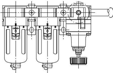
2. Do not allow twisting or bending moment to be applied other than the weight of the equipment itself.
