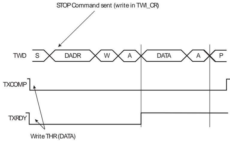
**Figure 40-7. Master Write with Multiple Data Bytes**
