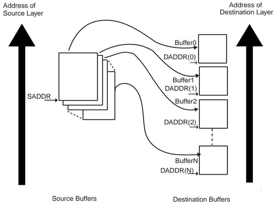
The DMAC Transfer flow is shown in [Figure 31-13 on page 531](#).
