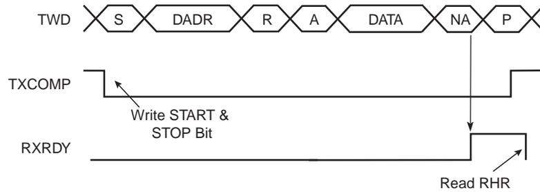
**Figure 40-10. Master Read with Multiple Data Bytes**
