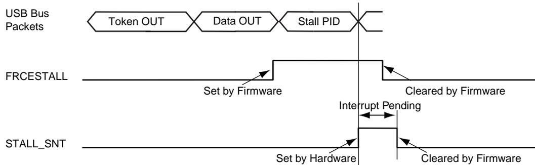
**Figure 34-18. Stall Handshake Data IN Transfer**
