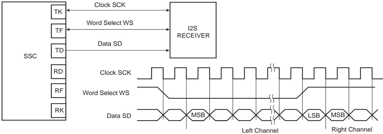
**Figure 41-18. Codec Application Block Diagram**
