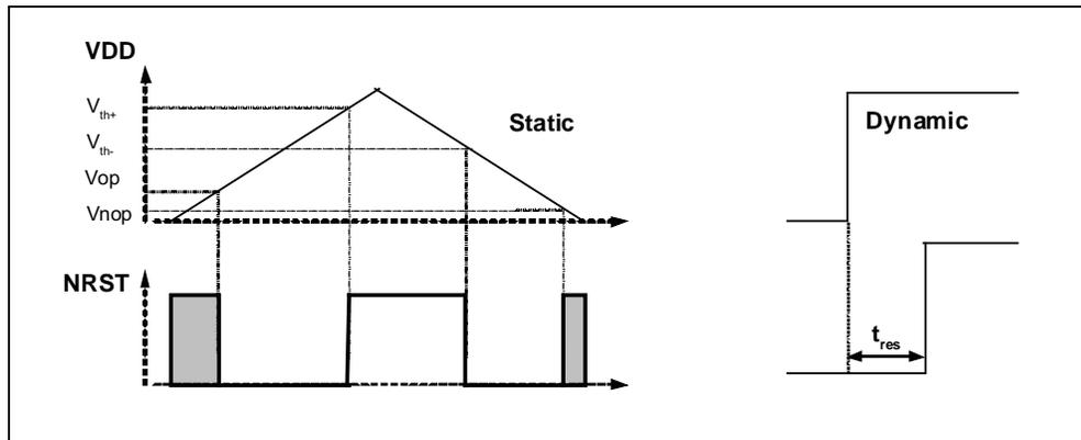
When a very slow (versus  $t_{RES}$ ) supply rising slope is applied on POR VDD pin, the reset time becomes negligible and the reset signal is released when VDD raises upper than  $V_{th+}$ .
