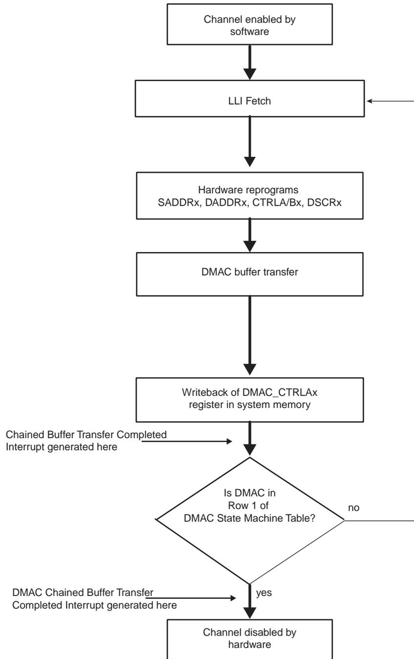
*Multi-buffer Transfer with Source Address Auto-reloaded and Destination Address Auto-reloaded (Row 10)*
