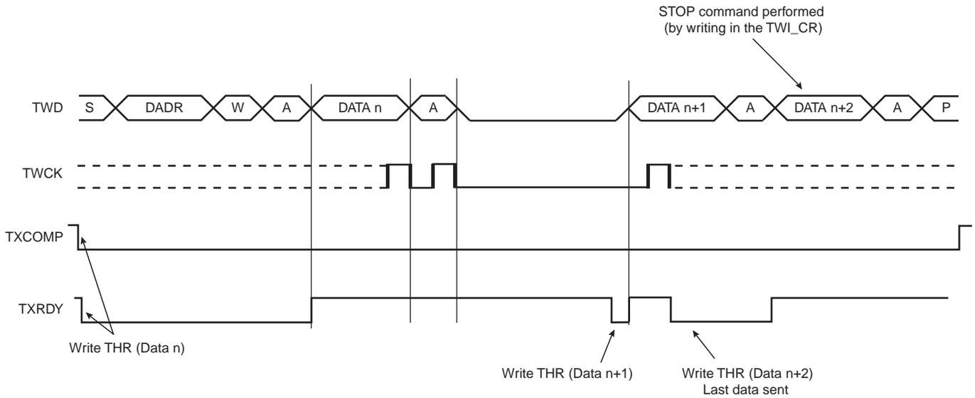
**Figure 40-8. Master Write with One Byte Internal Address and Multiple Data Bytes**
