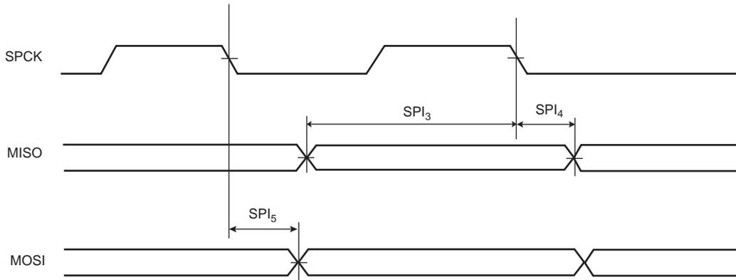
**Figure 54-11.SPI Slave Mode 0 and 3**
