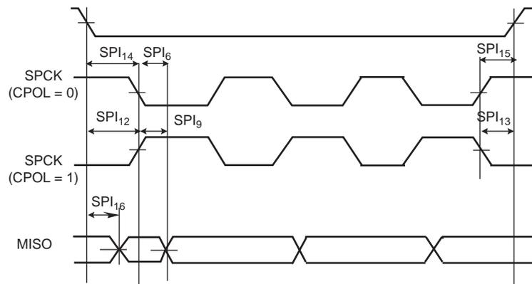
**Table 54-43. SPI Timings with 3v3 peripheral supply**
