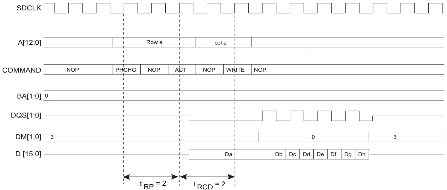
**Figure 29-5. Burst Write Access, Row Closed, DDR2-SDRAM Devices**
