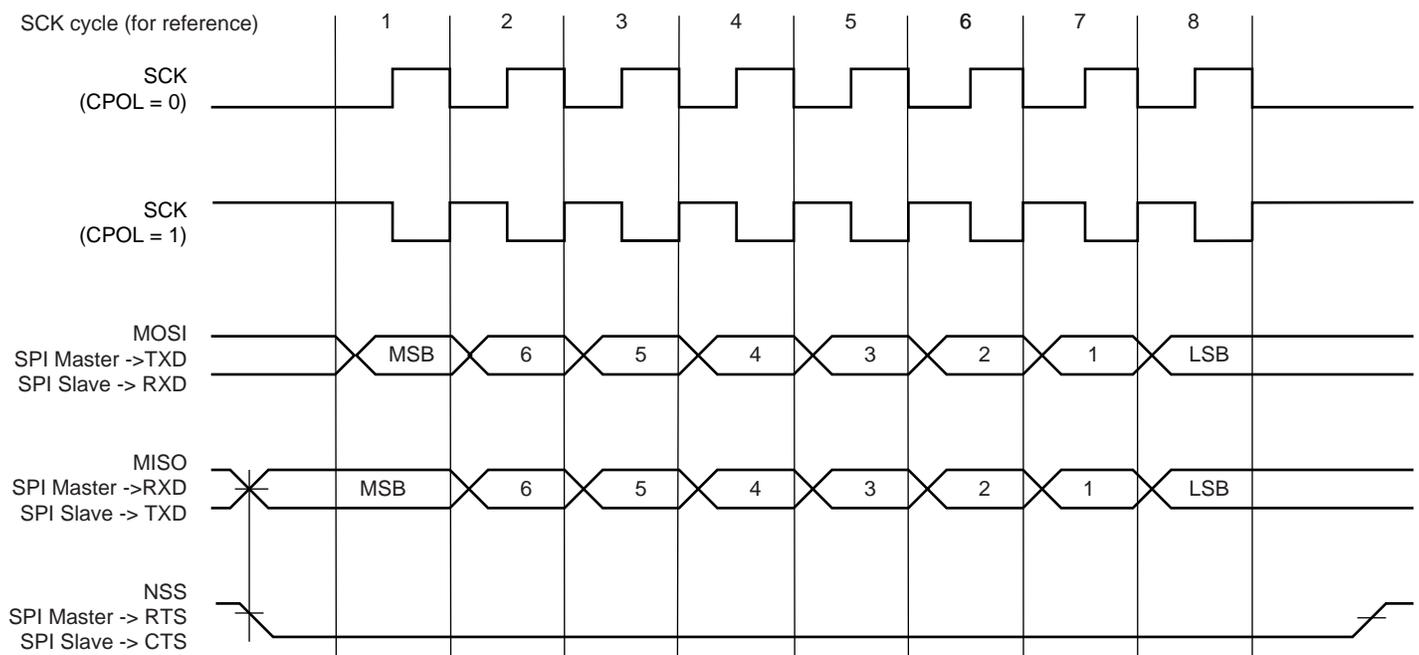
**Figure 44-38. SPI Transfer Format (CPHA = 0, 8 bits per transfer)**
