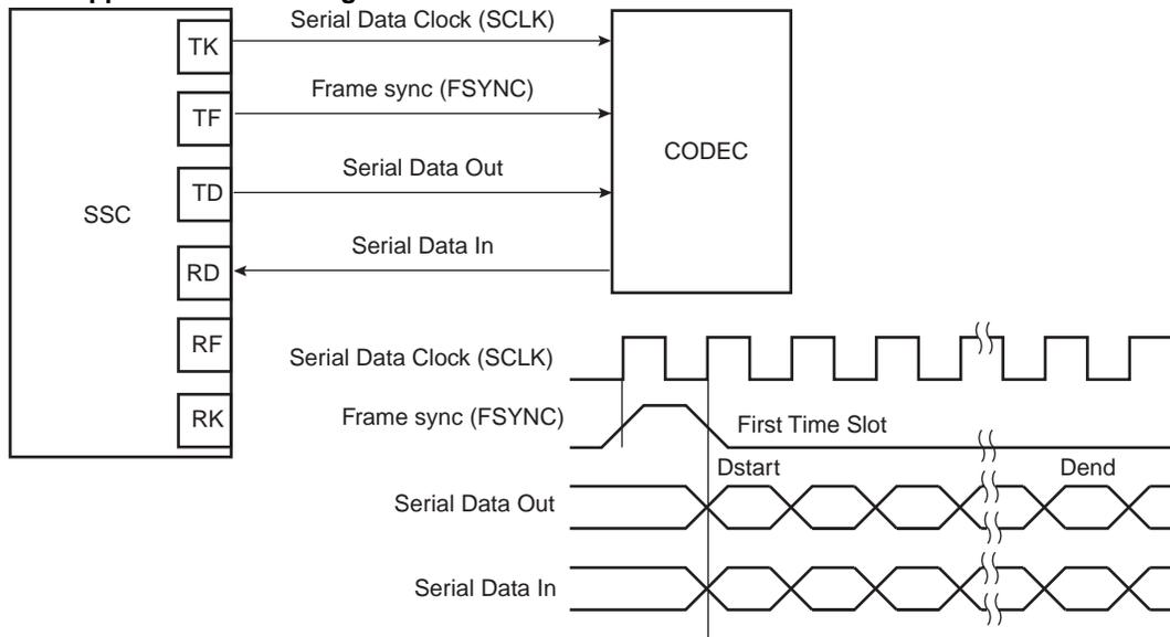
**Figure 41-19. Time Slot Application Block Diagram**
