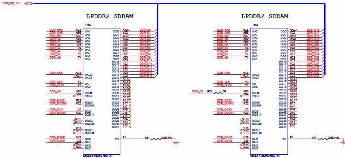
Cx LPDDR2 signals are to be connected as indicated in Table 28-3:
