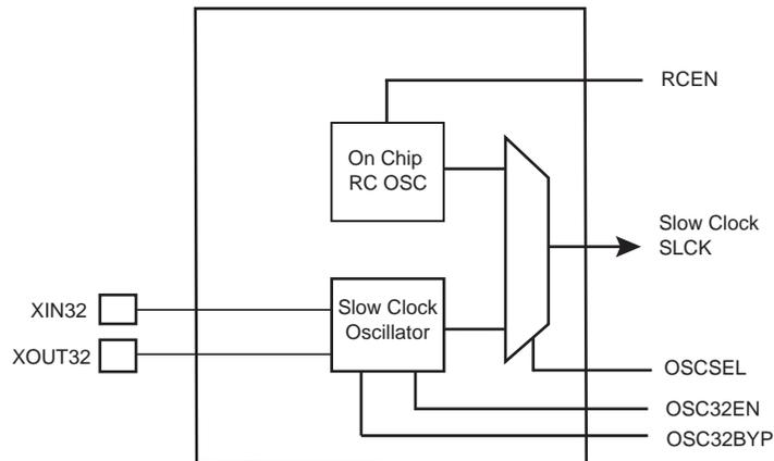
RCEN, OSC32EN, OSCSEL and OSC32BYP bits are located in the Slow Clock Controller Configuration Register (SCKC\_CR) located at the address 0xFFFFFE50 in the backed-up part of the System Controller and, thus, they are preserved while VDDBU is present.
