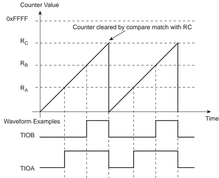
**Figure 47-11. WAVSEL = 10 with Trigger**
