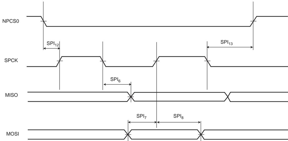
**Figure 54-12.SPI Slave Mode 1 and 2**
