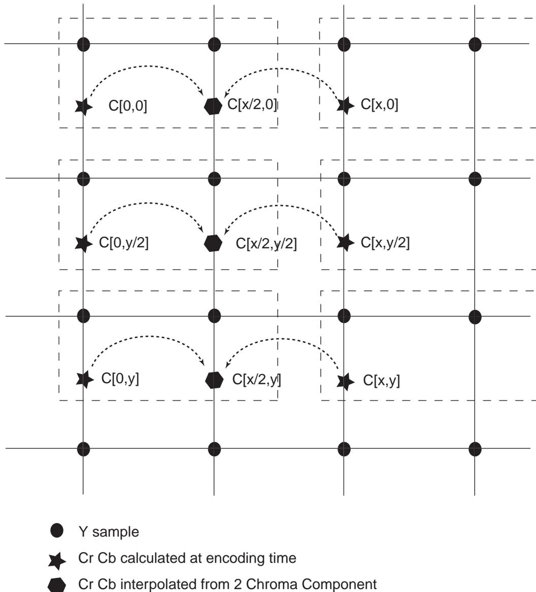
Figure 32-3. 4:2:2 Packed Upsampling Algorithm
