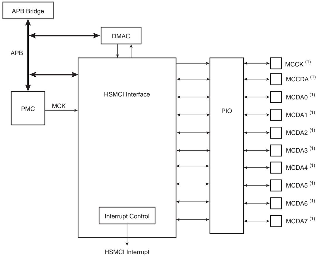
Note: 1. When several HSMCI (x HSMCI) are embedded in a product, MCCK refers to HSMCIx\_CK, MCCDA to HSMCIx\_CDA, MCDAy to HSMCIx\_Dy.
