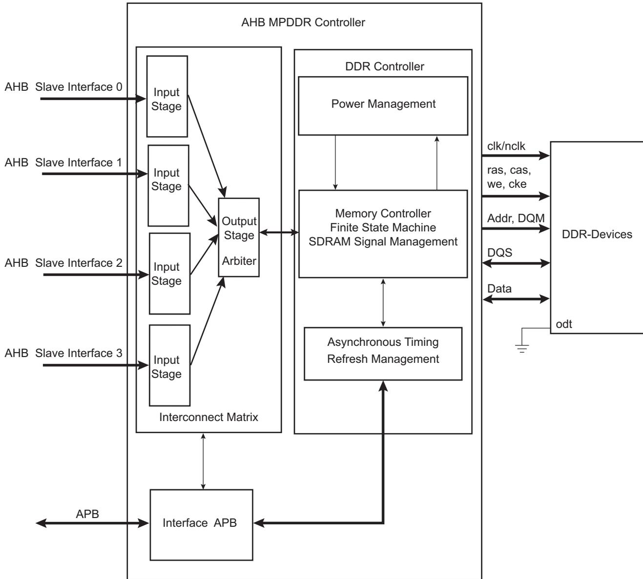
MPDDRC is partitioned in two blocks (see [Figure 29-1](#)):
