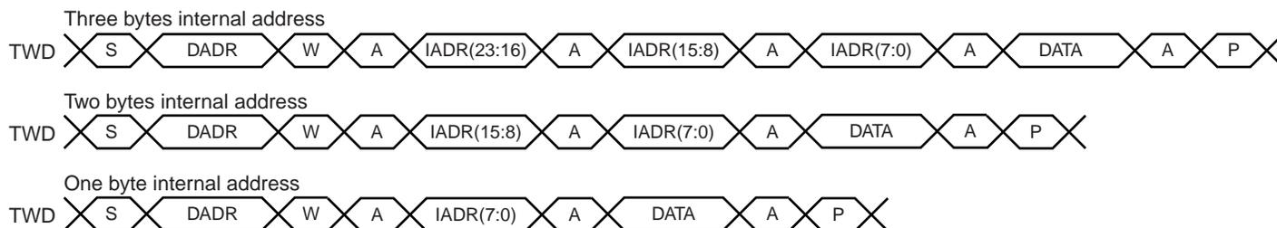
**Figure 40-13. Master Read with One, Two or Three Bytes Internal Address and One Data Byte**
