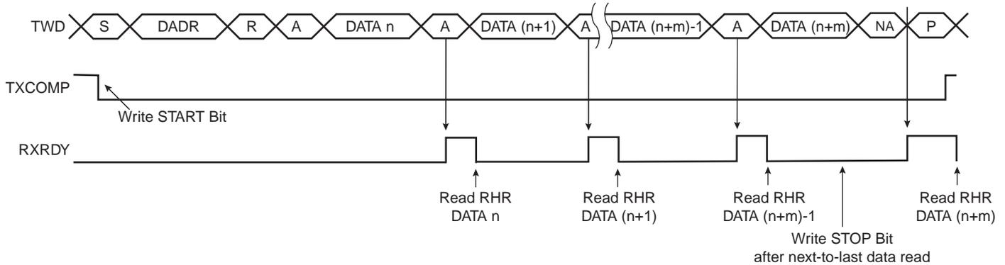
**Figure 40-11. Master Read Clock Stretching with Multiple Data Bytes**
