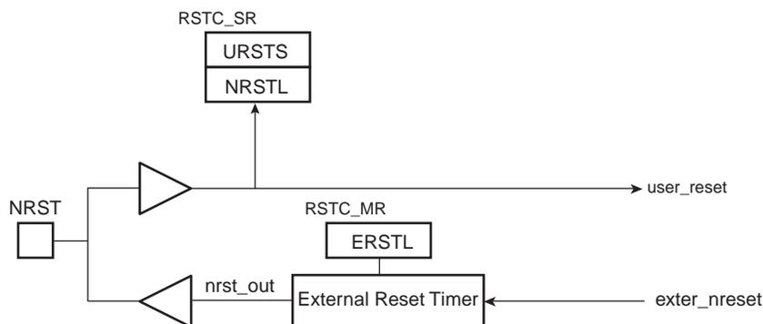
**NRST Signal** The NRST Manager handles the NRST input line asynchronously. When the line is low, a User Reset is immediately reported to the Reset State Manager. When the NRST goes from low to high, the internal reset is synchronized with the Slow Clock to provide a safe internal de-assertion of reset.
