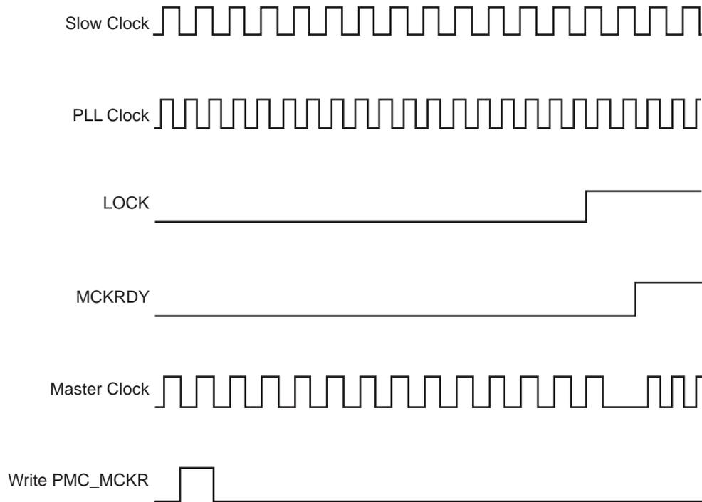
**Figure 26-10. Switch Master Clock from Main Clock to Slow Clock**
