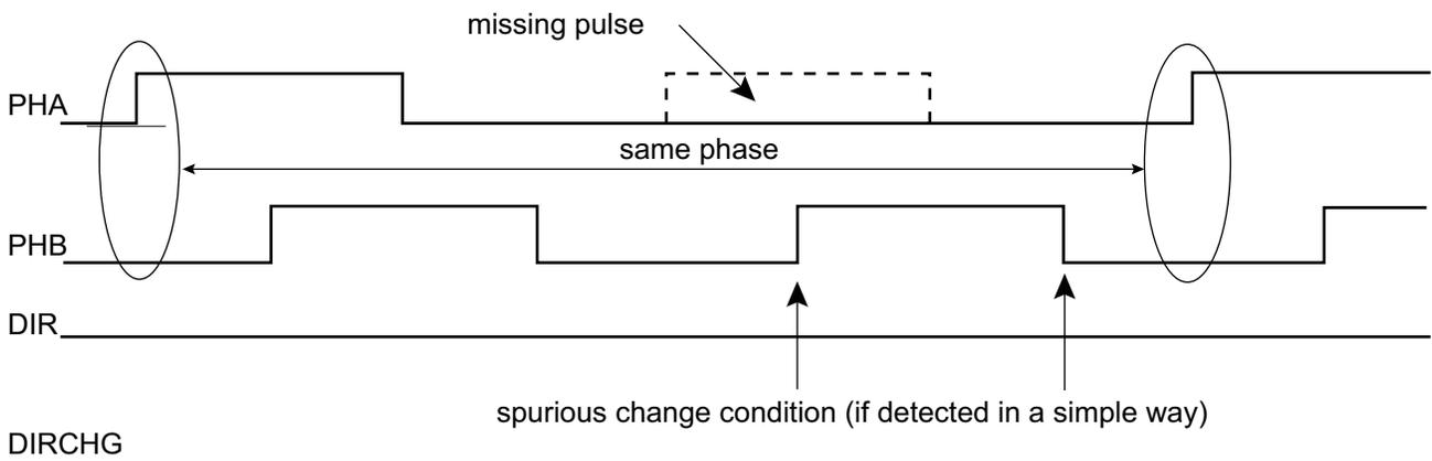
The direction change detection is disabled when QDTRANS is set in the TC\_BMR. In this case the DIR flag report must not be used.
