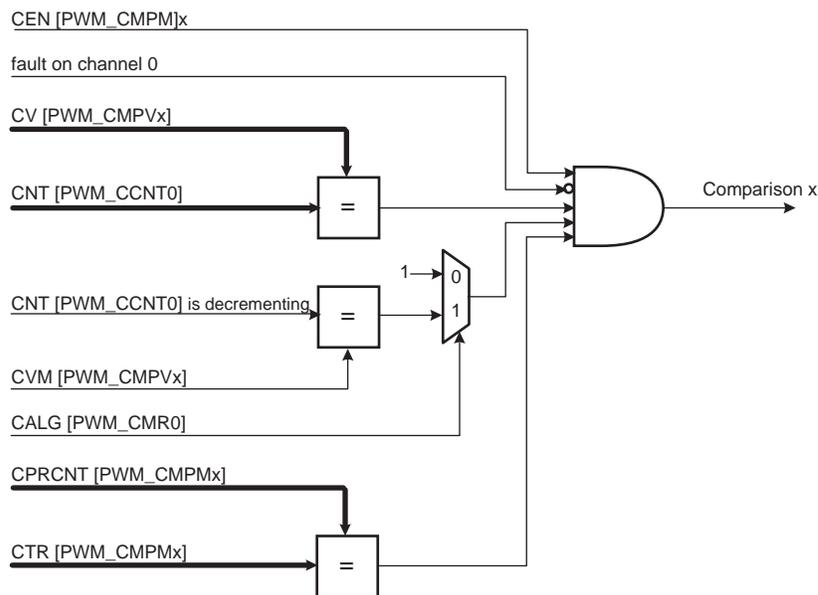
The comparison x matches when it is enabled by the bit CEN in the “[PWM Comparison x Mode Register](#)” (PWM\_CMPMx for the comparison x) and when the counter of the channel 0 reaches the comparison value defined by the field CV in “[PWM Comparison x Value Register](#)” (PWM\_CMPVx for the comparison x). If the counter of the channel 0 is center aligned (CALG = 1 in “[PWM Channel Mode Register](#)”), the bit CVM (in PWM\_CMPVx) defines if the
