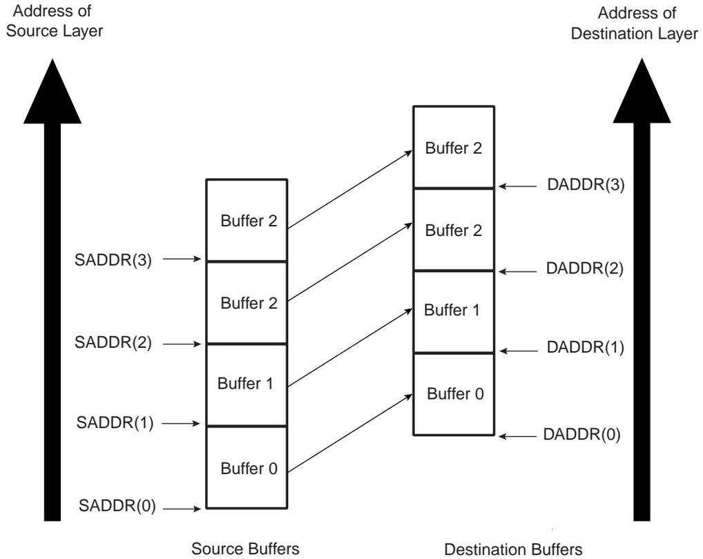
The DMAC transfer flow is shown in [Figure 31-9 on page 525](#).
