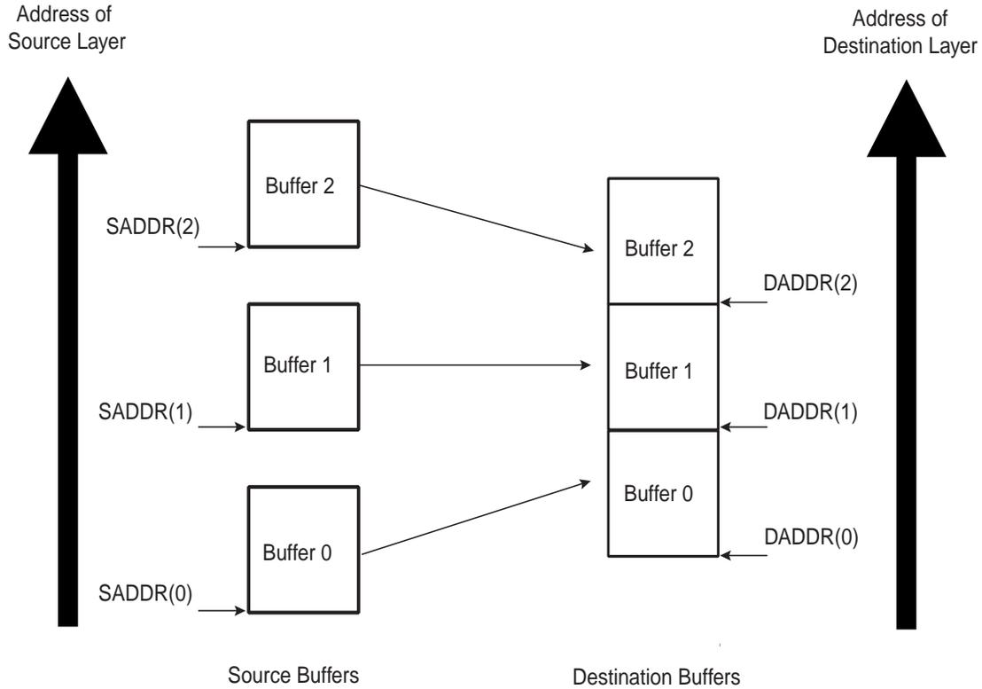
The DMAC transfer flow is shown in [Figure 31-17 on page 537](#).
