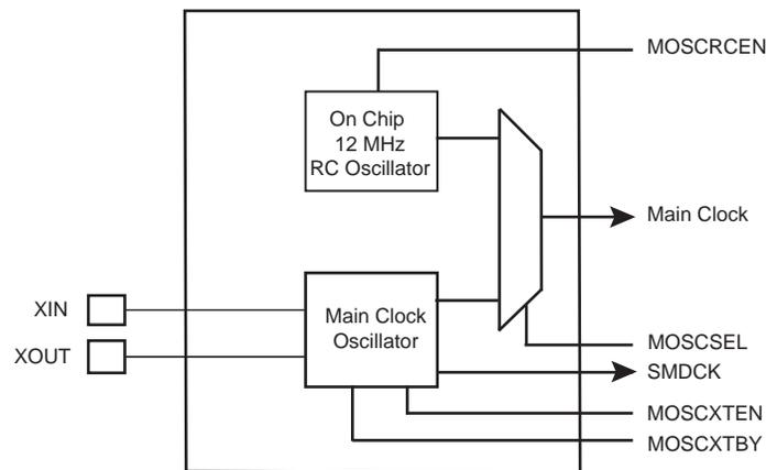
MOSCRGEN, MOSCXTEEN, MOSCSEL and MOSCXTBY bits are located in the PMC Clock Generator Main Oscillator Register (CKGR\_MOR).
