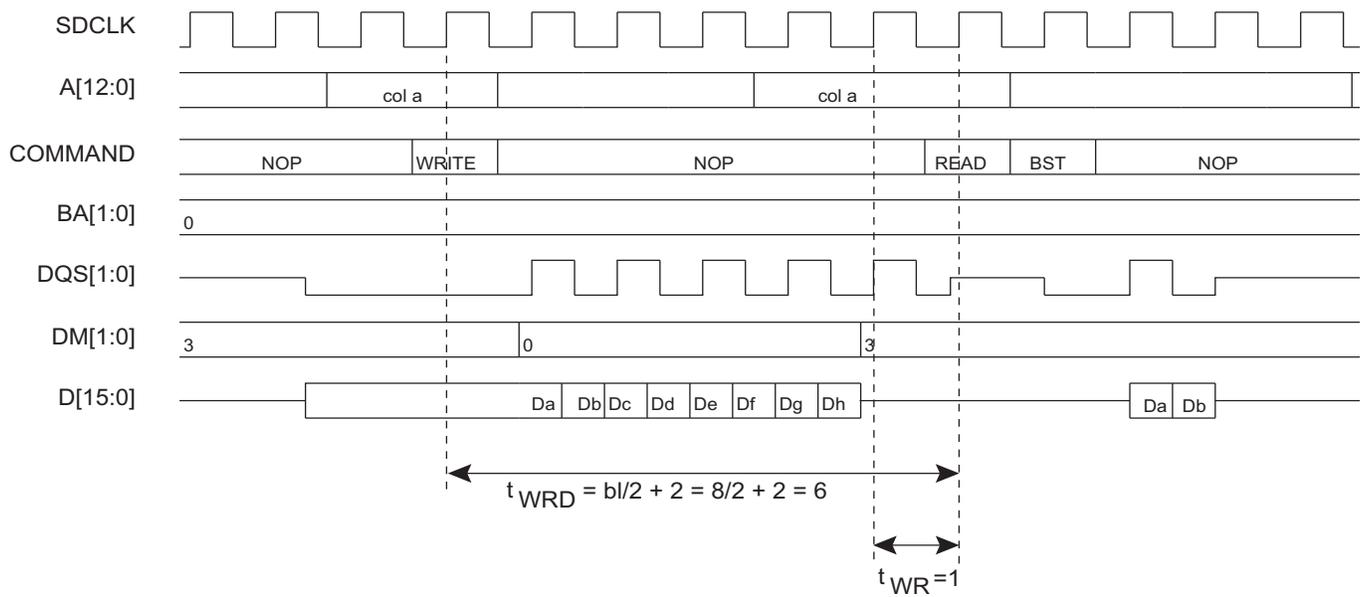
In case of a single write access, write operation should be interrupted by a read access but DM must be input 1 cycle prior to the read command to avoid writing invalid data. See [Figure 29-7 on page 360](#).
