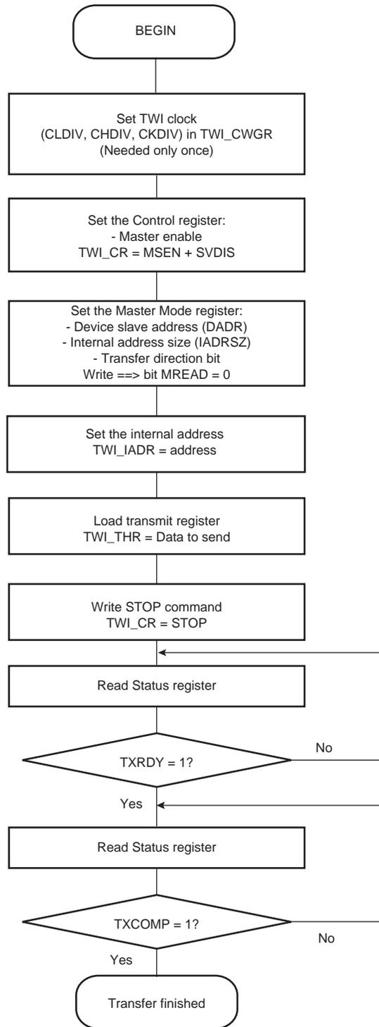
Figure 40-18. TWI Write Operation with Multiple Data Bytes with or without Internal Address
