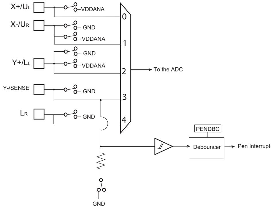
The Touchscreen Pen Detect can be used to generate an ADC interrupt to wake up the system. The Pen Detect generates two types of status, reported in the “ADC Interrupt Status Register”:
