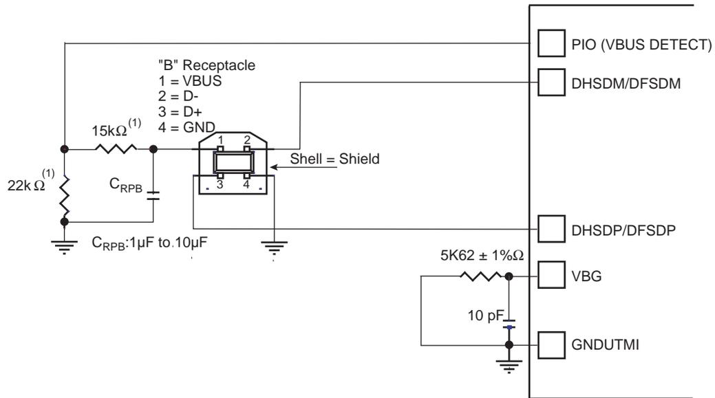
Note: The values shown on the 22 kΩ and 15 kΩ resistors are only valid with 3V3 supplied PIOs.
