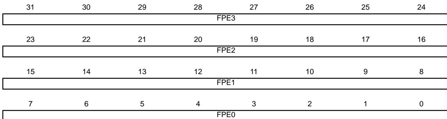
This register can only be written if bits WPSWS5 and WPHWS5 are cleared in the [“PWM Write Protection Status Register”](#) .
