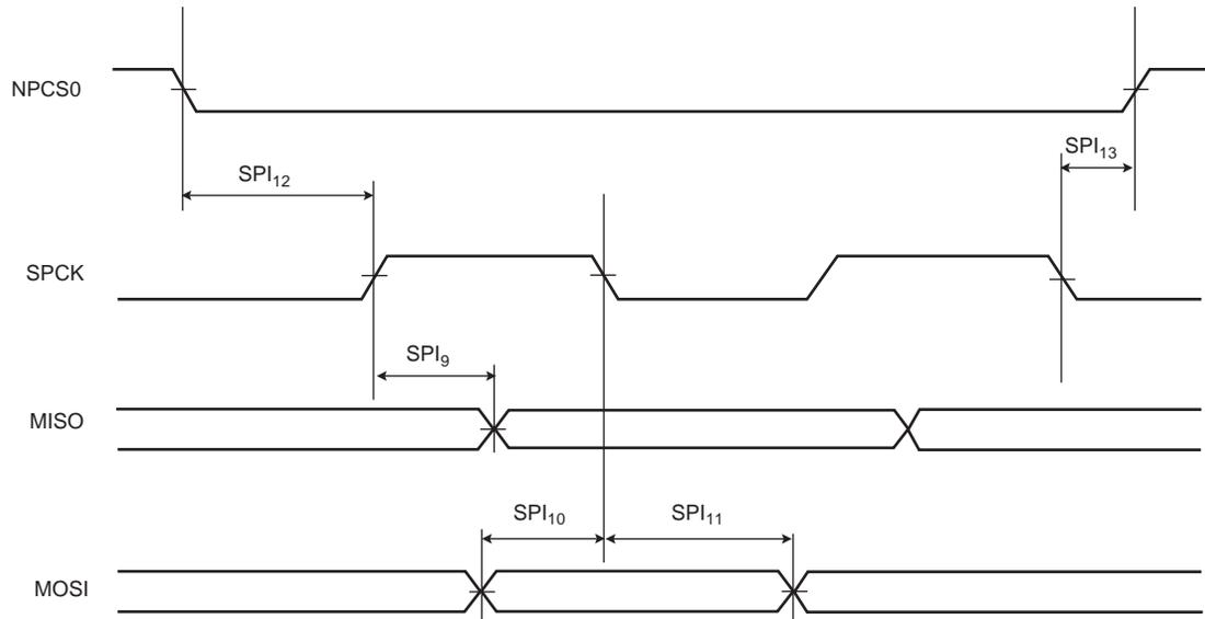
**Figure 54-13.SPI Slave Mode - NPCS Timings**
