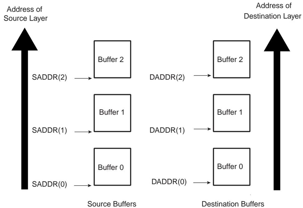
If the user needs to execute a DMAC transfer where the source and destination address are contiguous but the amount of data to be transferred is greater than the maximum buffer size `DMAC_CTRLAx.BTSIZE`, then this can be achieved using the type of multi-buffer transfer as shown in [Figure 31-8 on page 524](#).
