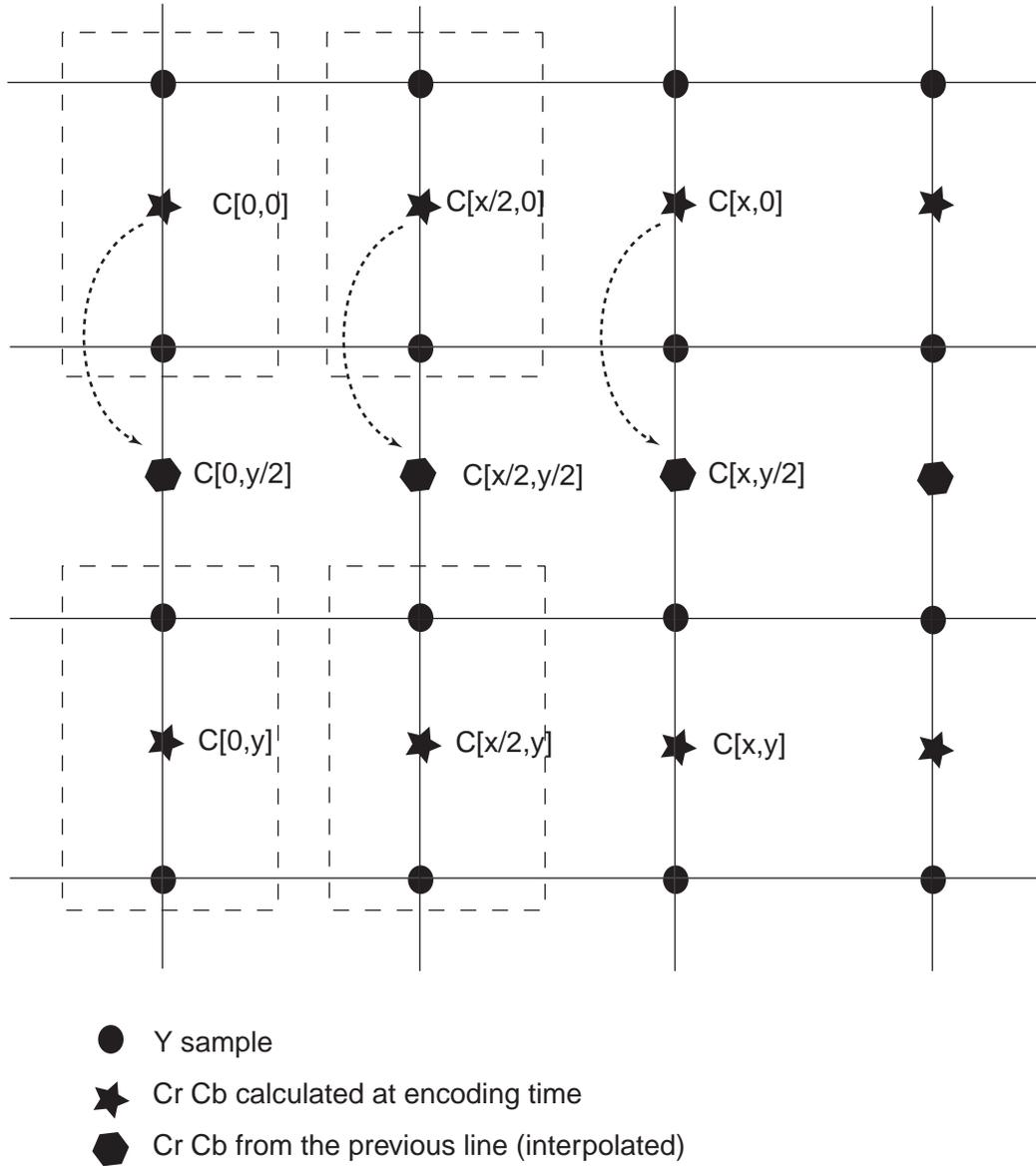
Figure 32-4. 4:2:2 Semiplanar and Planar Upsampling Algorithm - 90 or 270 Degree Rotation Activated
