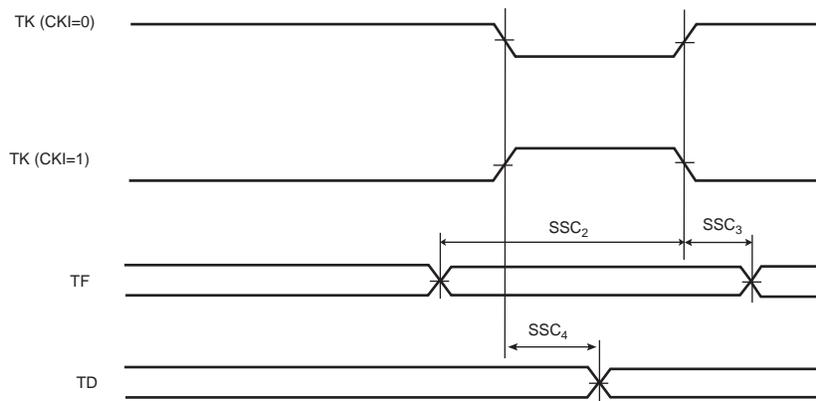
Figure 54-19.SSC Transmitter, TK and TF in Input
