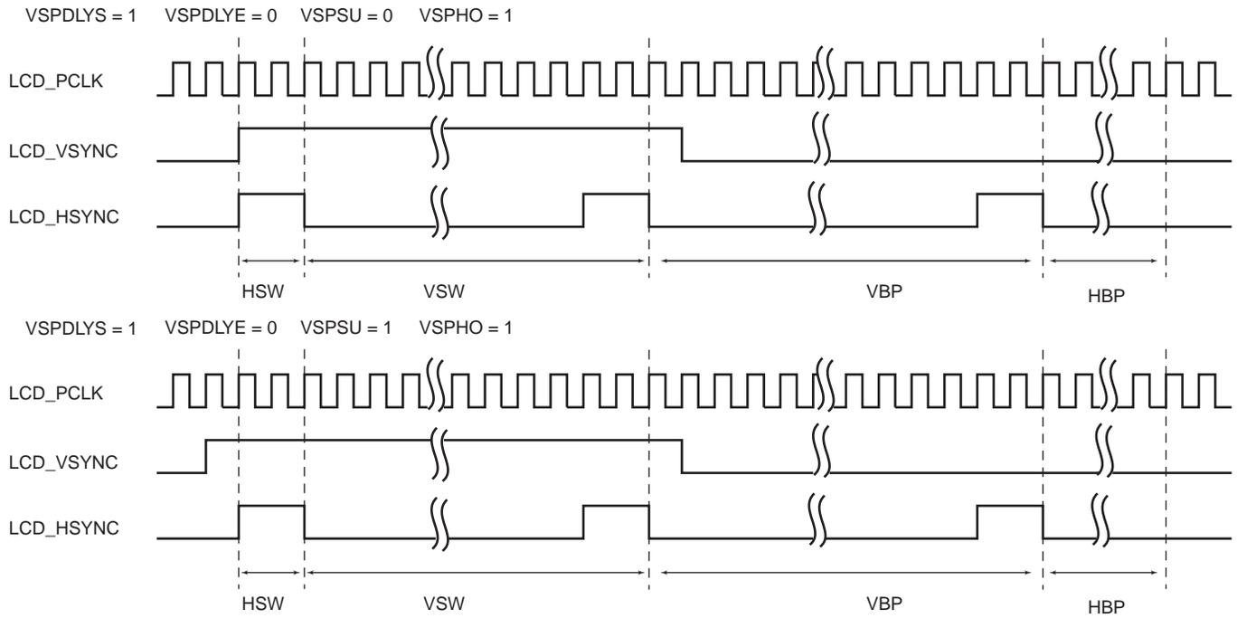
**Figure 32-18.DISP Signal Timing Diagram**
