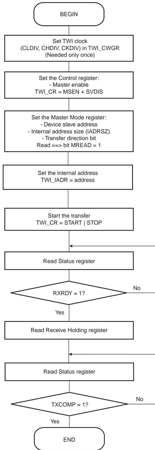
Figure 40-21. TWI Read Operation with Multiple Data Bytes with or without Internal Address
