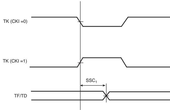
Figure 54-18.SSC Transmitter, TK in Output and TF in Input
