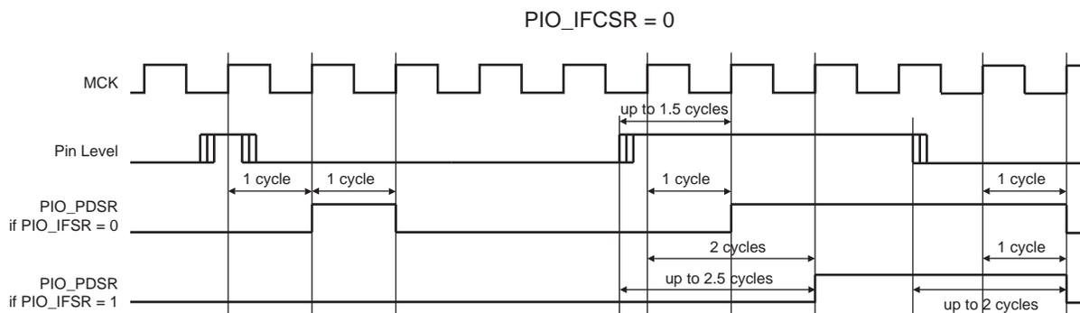
**Figure 27-6. Input Debouncing Filter Timing**
