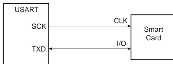
When operating in ISO7816, either in T = 0 or T = 1 modes, the character format is fixed. The configuration is 8 data bits, even parity and 1 or 2 stop bits, regardless of the values programmed in the CHRL, MODE9, PAR and CHMODE fields. MSBF can be used to transmit LSB or MSB first. Parity Bit (PAR) can be used to transmit in normal or inverse mode. Refer to “[USART Mode Register](#)” on page 1407 and “[PAR: Parity Type](#)” on page 1408.
