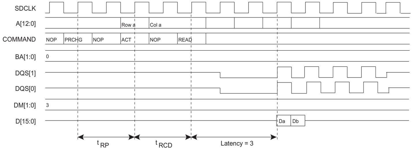
**Figure 29-11. Burst Read Access, Latency = 2, DDR-SDRAM Devices**
