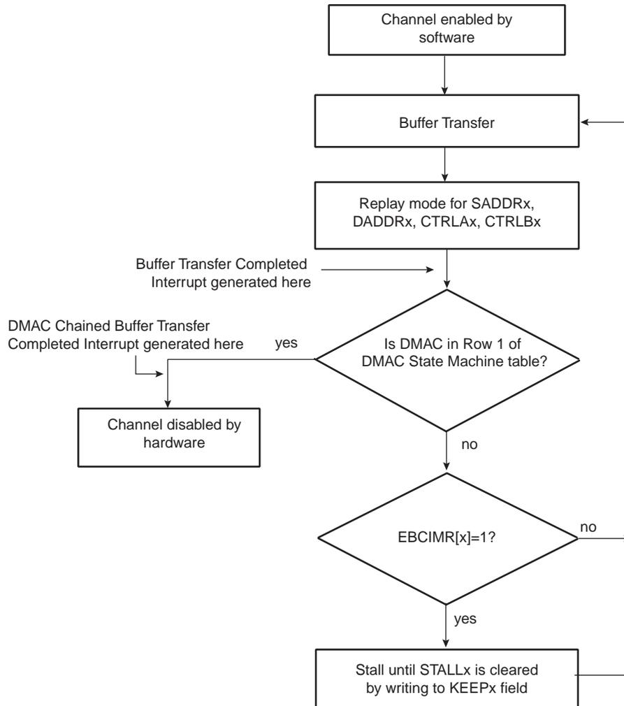
*Multi-buffer Transfer with Source Address Auto-reloaded and Linked List Destination Address (Row 6)*
