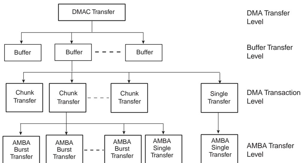
**Figure 31-3. DMAC Transfer Hierarchy for Memory**
