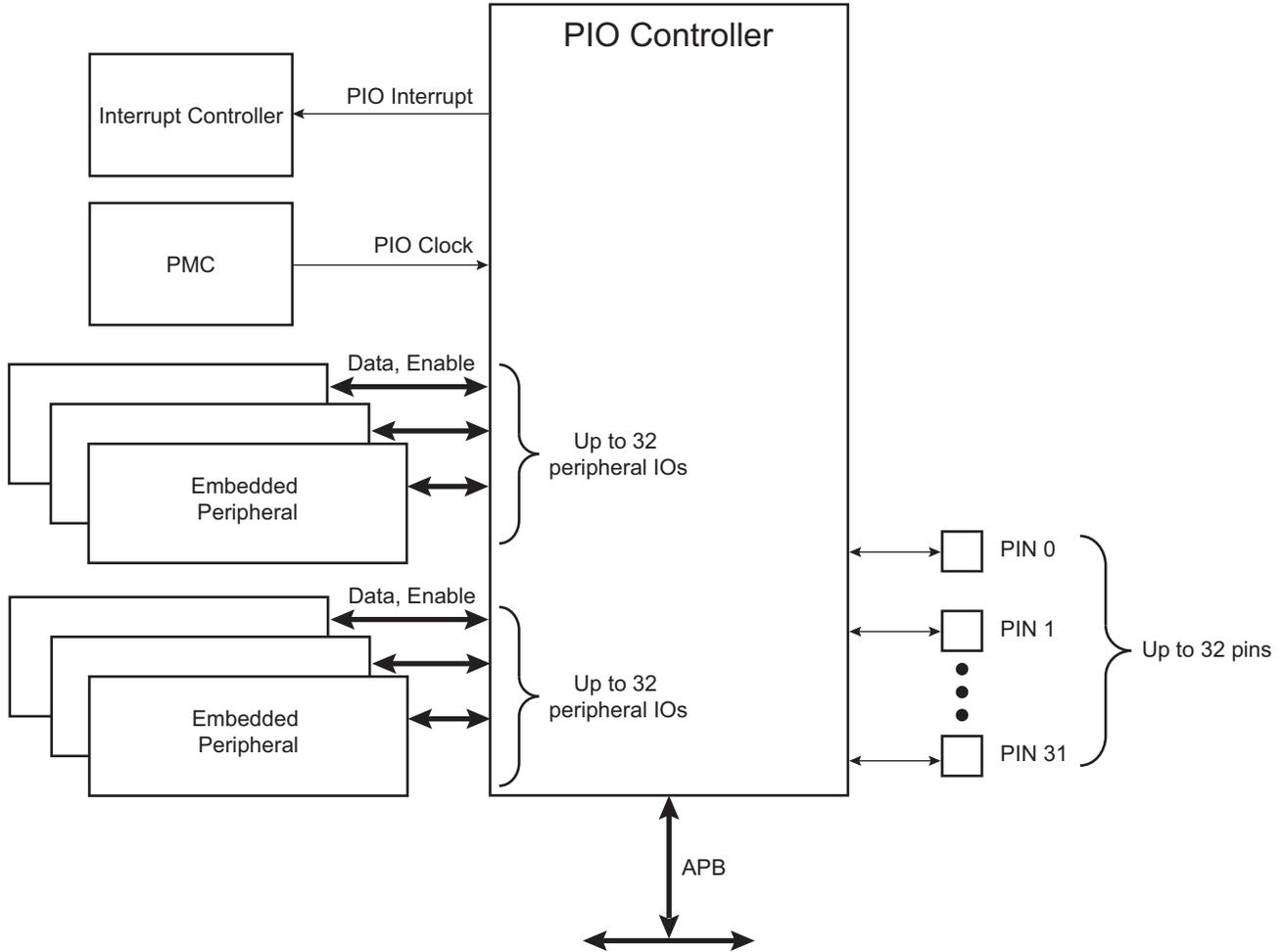
Figure 27-2. Application Block Diagram
