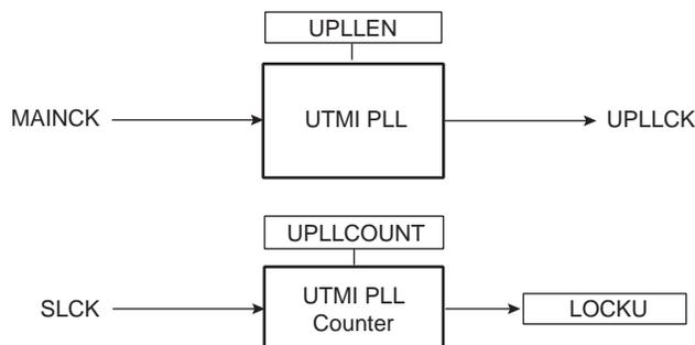
Whenever the UTMI PLL is enabled by writing UPLEN in CKGR\_UCKR, the LOCKU bit in PMC\_SR is automatically cleared. The values written in the PLLCOUNT field in CKGR\_UCKR are loaded in the UTMI PLL counter. The UTMI PLL counter then decrements at the speed of the Slow Clock divided by 8 until it reaches 0. At this time, the LOCKU bit is set
