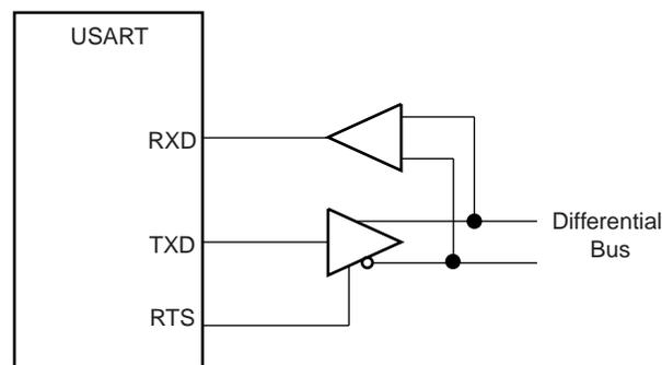
The USART is set in RS485 mode by writing the value 0x1 to the USART\_MODE field in the Mode Register (US\_MR). The RTS pin is at a level inverse to the TXEMPTY bit. Significantly, the RTS pin remains high when a timeguard is programmed so that the line can remain driven after the last character completion. Figure 44-36 gives an example of the RTS waveform during a character transmission when the timeguard is enabled.
