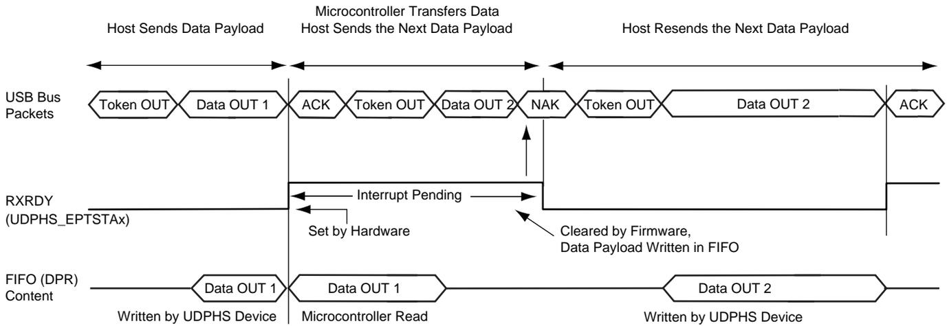
**Figure 34-15. Data OUT Transfer for an Endpoint with Two Banks**
