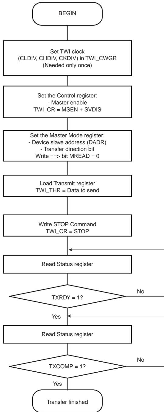
Figure 40-17. TWI Write Operation with Single Data Byte and Internal Address
