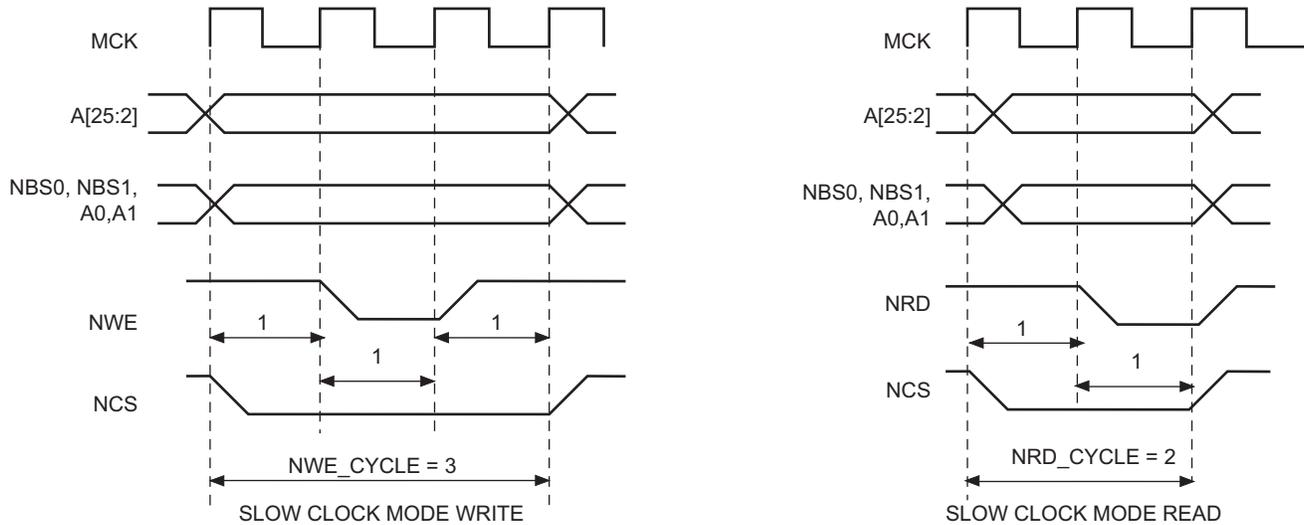
Table 30-7. Read and Write Timing Parameters in Slow Clock Mode
