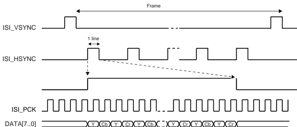
Figure 33-4. SAV and EAV Sequence Synchronization
