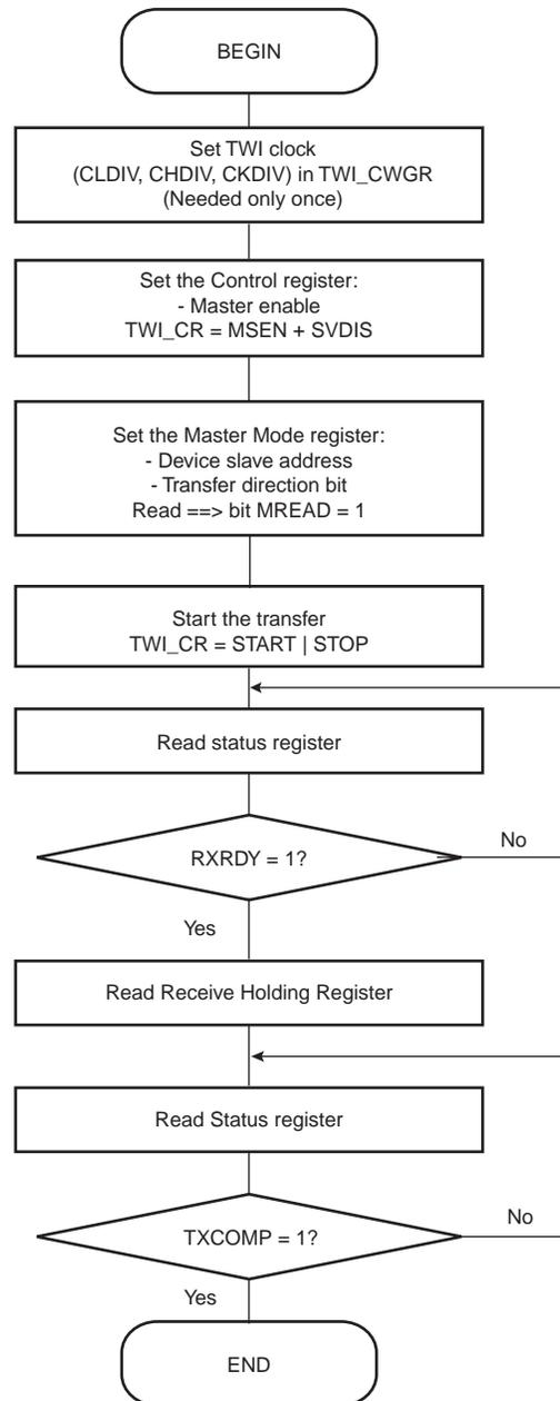
Figure 40-20. TWI Read Operation with Single Data Byte and Internal Address
