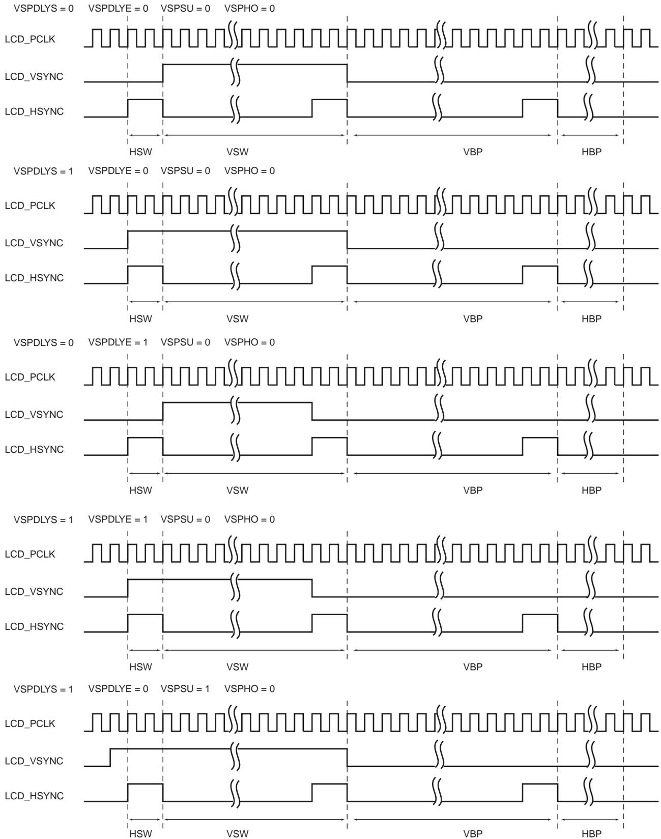
**Figure 32-17. Vertical Synchronization Timing (part 2)**
