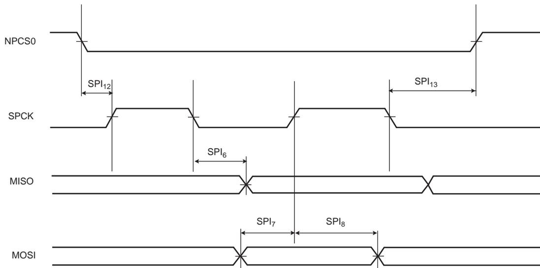
Figure 54-31. SPI Slave mode - NPCS timings
