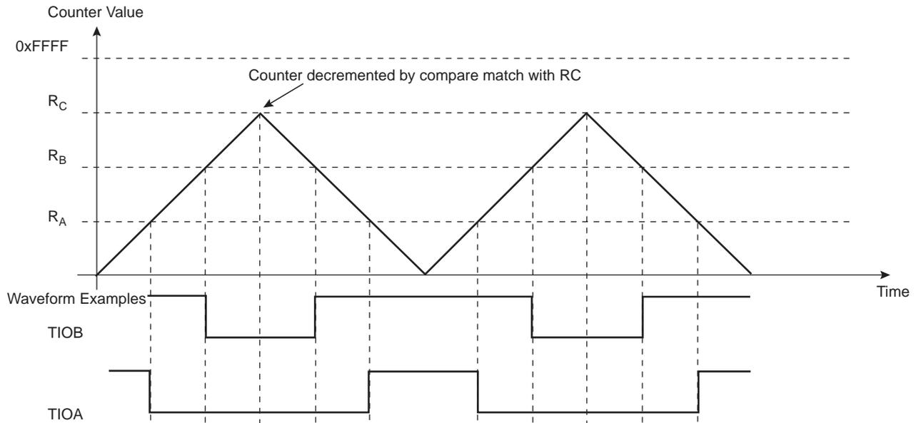
**Figure 47-15. WAVSEL = 11 with Trigger**
