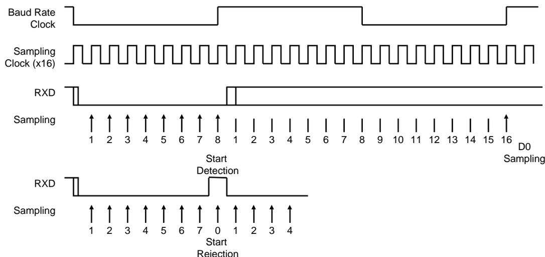
**Figure 44-13. Asynchronous Character Reception**
