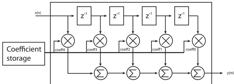
**Figure 32-8. Vertical Resampler Filter Architecture**
