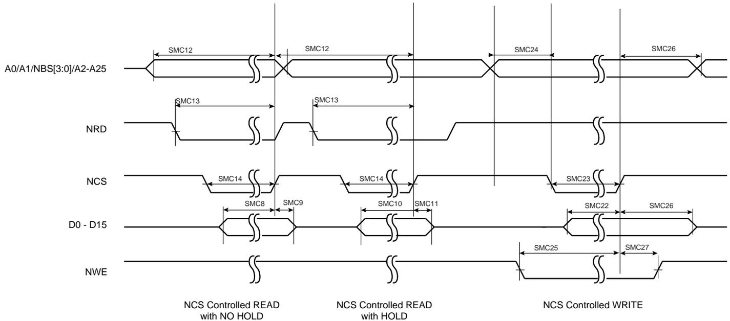
**Figure 54-7. SMC Timings - NRD Controlled Read and NWE Controlled Write**
