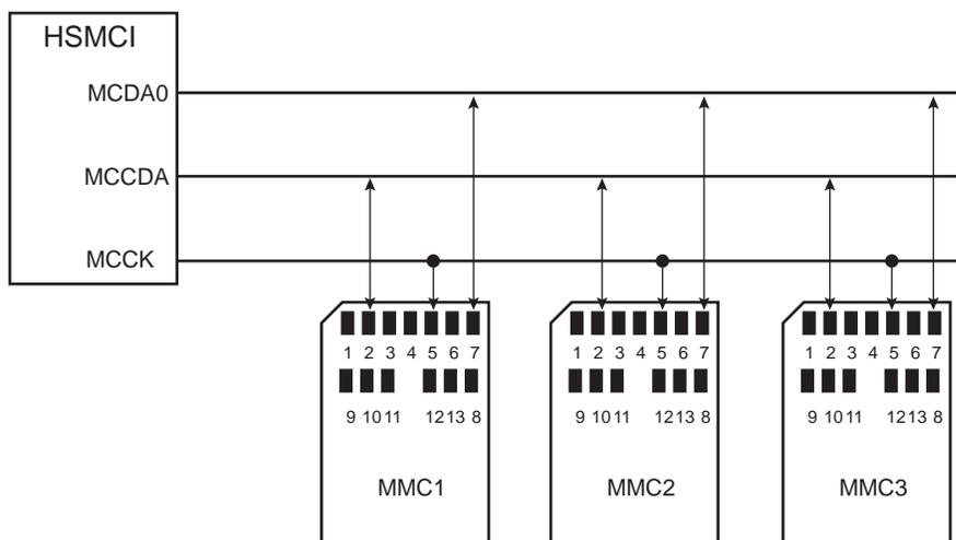
Note: When several HSMCI (x HSMCI) are embedded in a product, MCCK refers to HSMCIx\_CK, MCCDA to HSMCIx\_CDA, MCCDB to HSMCIx\_CDB, MCDAy to HSMCIx\_DAy, MCDBy to HSMCIx\_DBy.
