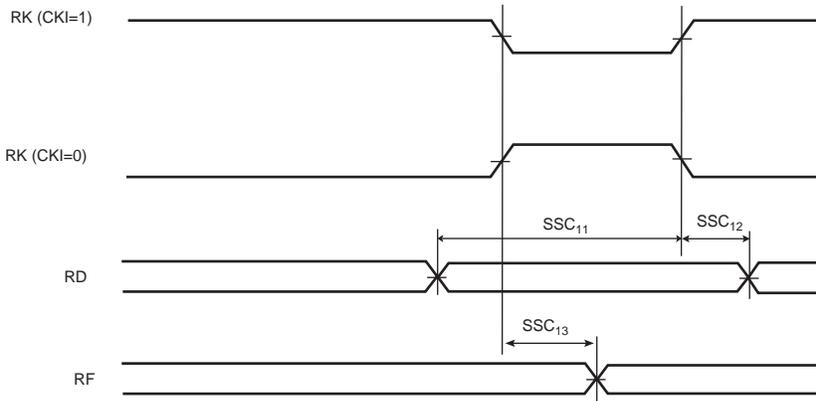
**Figure 54-23.SSC Receiver, RK in Output and RF in Input**
