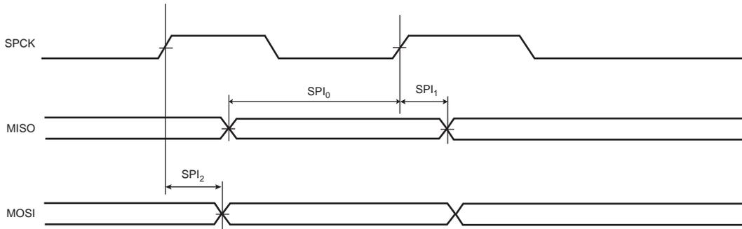
**Figure 54-10. SPI Master mode 0 and 3**
