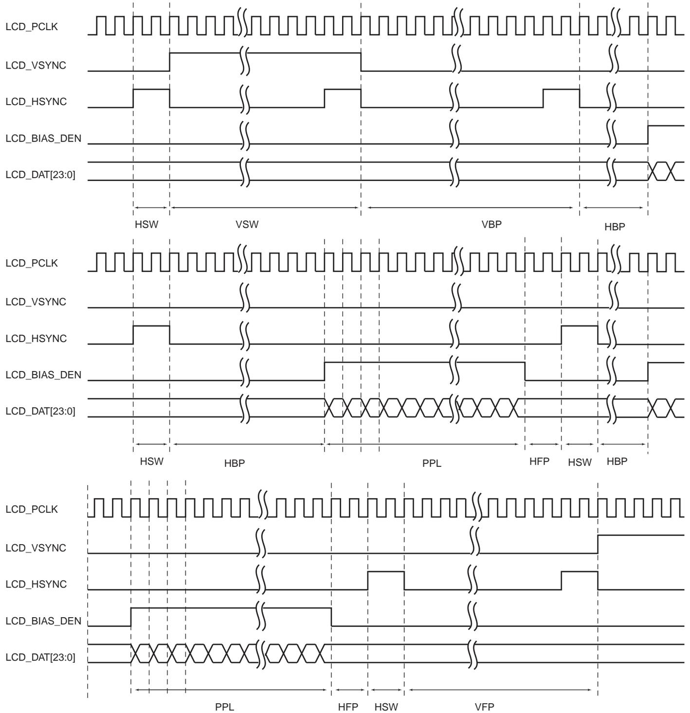
**Figure 32-16. Vertical Synchronization Timing (part 1)**
