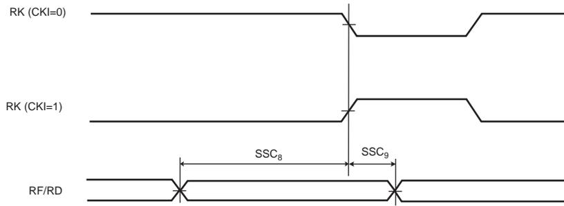
**Figure 54-21.SSC Receiver, RK in Input and RF in Output**
