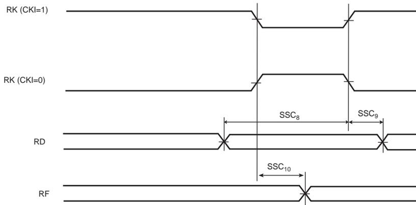
**Figure 54-22.SSC Receiver, RK and RF in Output**
