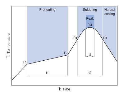
Preheating Soldering Peak Temp. Time Temp. Time Temp. Time T1 T2 **T4** Т3 t3 150°C 180°C 60 to 120s 220°C 40s 260°C 5s
