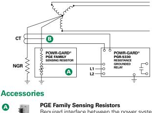
Required interface between the power system and the PGR-5330. Eliminates hazardous voltage levels at the relay.
