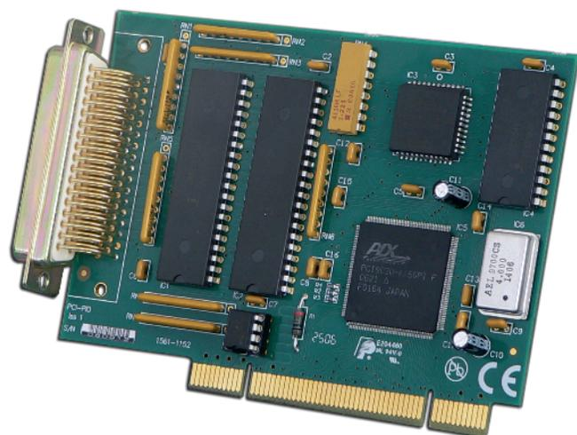
The PCI-PIO is a PCI-compatible half-card which provides digital input/outputs and counter/timers. There are 48 TTL-compatible programmable digital input/outputs available from the board. If the controlling devices are used in handshake mode, the handshake lines are available as interrupt sources.
