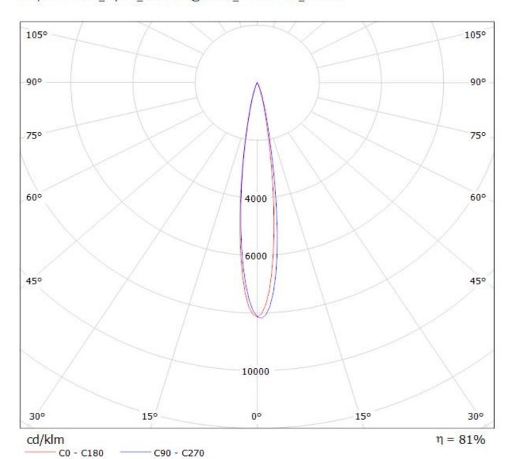
Luminaire: LEDiL Oy FC14972\_FLORENTINA-2X2-D\_(NVSxx19c) Lamps: 1 x NVSxx19c\_412.136Im@250mA\_P=2.81612W\_I=0.250A
