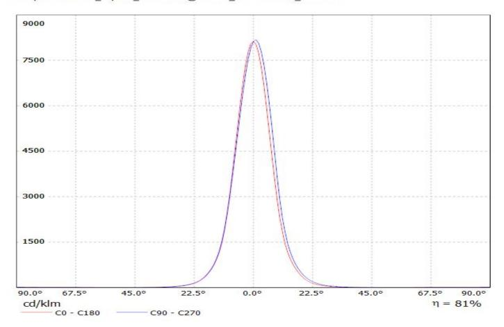
Luminaire: LEDiL Oy FC14972\_FLORENTINA-2X2-D\_(NVSxx19c) Lamps: 1 x NVSxx19c\_412.136Im@250mA\_P=2.81612W\_I=0.250A
