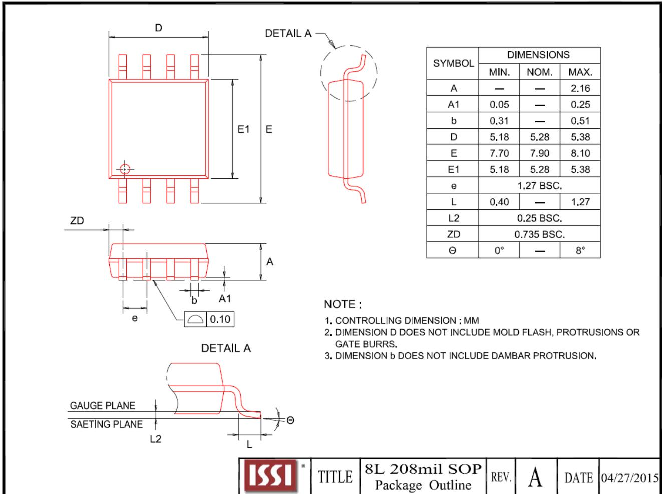
**Note: All dimensions are in millimeters. Lead co-planarity is 0.1mm.**
