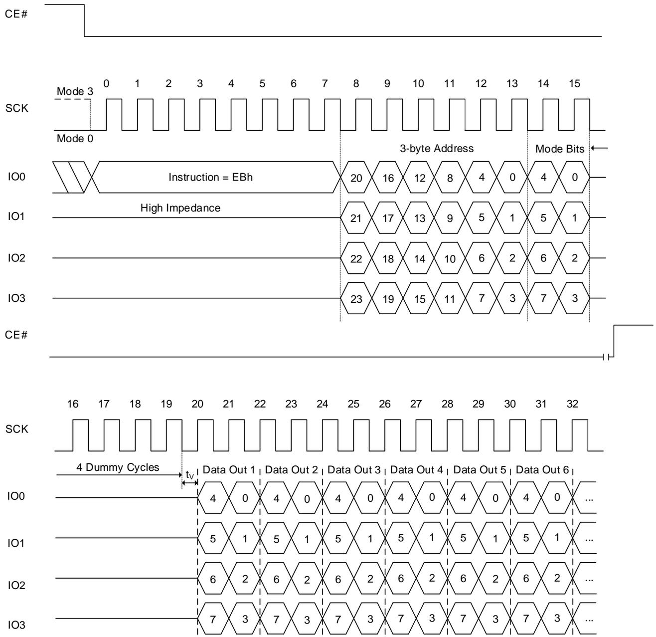
**Note:** If the mode bits=AXh (X: don't care), it can execute the AX read mode (without command). Anything but AXh in the mode byte cycle will exit the AX read mode.
