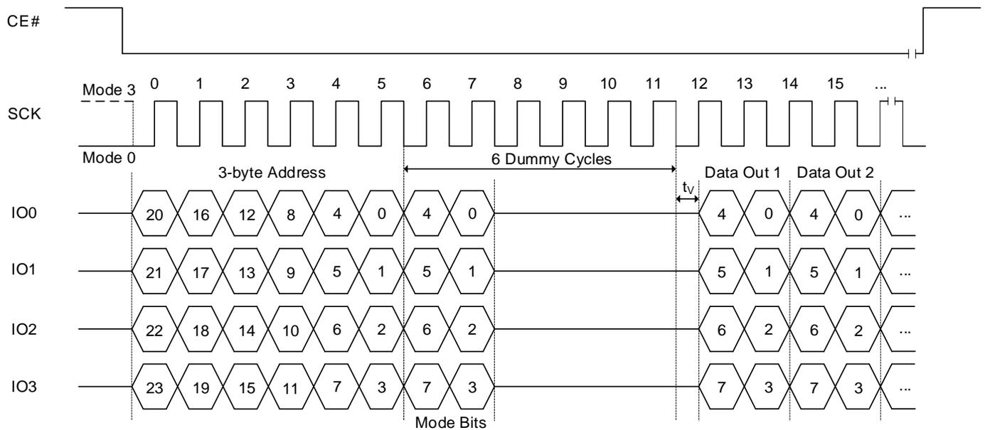
**Note: If the mode bits=AXh (X: don't care), it can execute the AX read mode (without command). Anything but AXh in the mode byte cycle will exit the AX read mode.**
