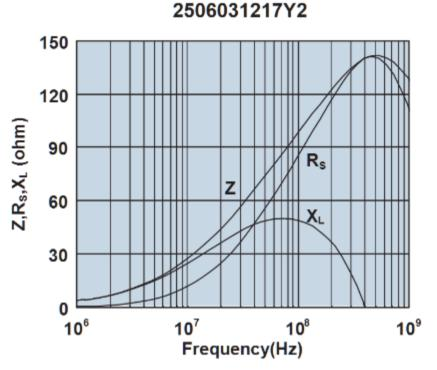
Impedance, reactance, and resistance vs. frequency.
