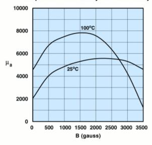
Measured on an 18/10/6mm toroid at 10kHz.
