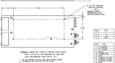
DO NOT EXCEED 30 INCH-LBS (MAX TORQUE) WHEN TIGHTENING TOP NUTS ON OUTPUT STUDS.
