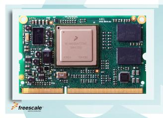
AXEL LITE enables designers to create smart products suitable for harsh mechanical and thermal environments, allowing for the development of high computing and reliable solutions.
