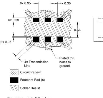
Dimensions are in Millimeters Mounting Footprint
