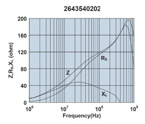
Impedance, reactance, and resistance vs. frequency.
