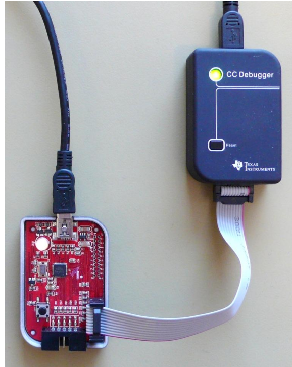
Figure 16 - Programming the bootloader on the CC Debugger using another CC Debugger
