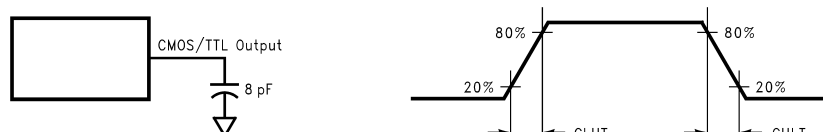
Figure 6. DS90CF384A/DS90CF364A (Receiver) CMOS/TTL Output Load and Transition Times
