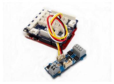
1. Connect the Grove socket marked "IN" on the LED Strip Driver and digital port 2 on the Base Shield with a Grove cable.
