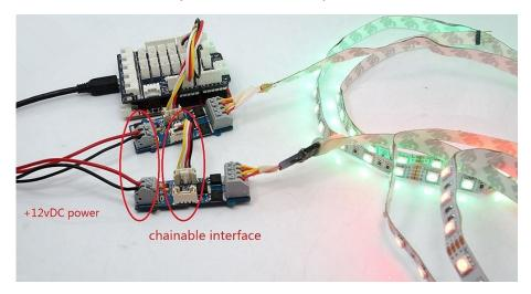
In cases that you want to utilize the cascade feature, prepare another driver and strip first. Then use a Grove cable to connect the Grove socket marked "out" on the first board and the Grove socket marked "IN" on the second board. Done. Two strips will shine in sync now.
