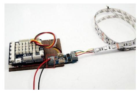
3. Connect the 12V DC or 9V DC power wires to the 2 pin terminal.
