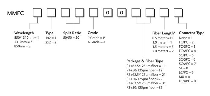
\* The tolerance of fiber length is +/-0.1m. 1 meter is standard. The lead time for special fiber length will be longer.
