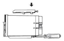
After attaching the mounting brackets, turn the screws clockwise to tighten them sufficiently. When the screws are completely tightened, you will hear the threads disengage.
