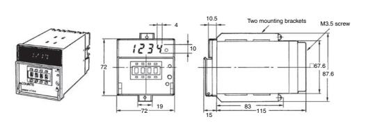
Note: 1. The panel cutouts for the H7AN are as shown (according to DIN437000).
