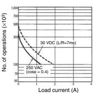
Reference: 0.15 A max. can be switched 100,000 times at 125 VDC ( $\cos\phi = 1$ ).
