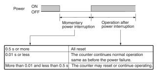
Note: Use a model with a backup function (models ending in "-M") to maintain the settings even for power interruptions. Be sure to enable the backup function.
