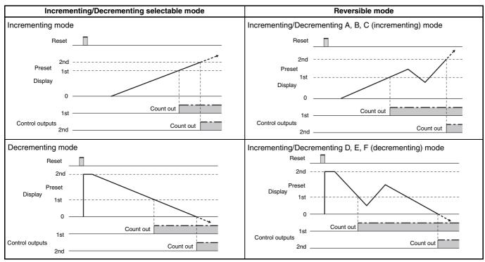
Note: Two-stage counters, set the counters so that the interval between 1st and 2nd count out will be more than 5 ms. For Incrementing/
