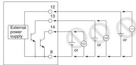
When using heaters, be sure to use a thermal switch for the load circuit.
