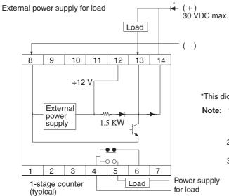
\*This diode is necessary if the supply voltage is below 12 V.
