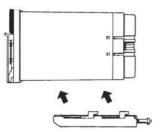
Turn the screws on the mounting brackets counterclockwise to loosen them sufficiently. Attach the bottom mounting bracket first.
