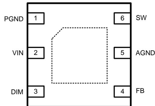
**Figure 2. Pinout**
