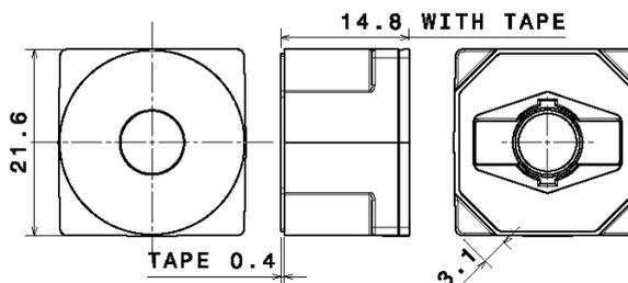
Space for D=5.0 mm screw head between the lenses for fastening of PCB
