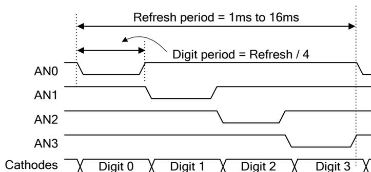
Figure 19. Four digit scanning display controller timing diagram.
