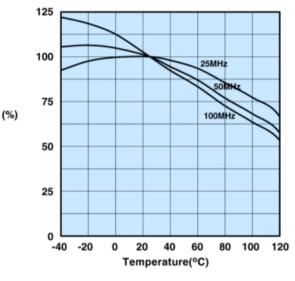
Measured on a 2643000301 using the HP4291A.
