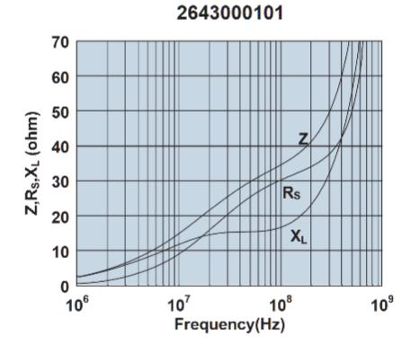
Impedance, reactance, and resistance vs. frequency.
