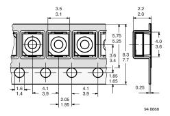
Fig. 10 - Tape Dimensions in mm for PLCC-2
