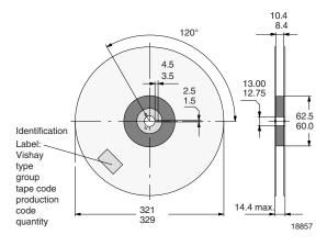
Fig. 13 - Dimensions of Reel-GS18
