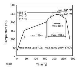
Fig. 8 - Lead (Pb)-free Reflow Solder Profile acc. J-STD-020
