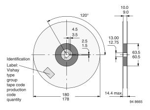
Fig. 12 - Dimensions of Reel-GS08
