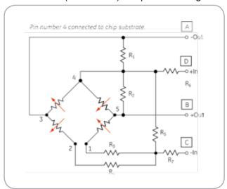
NPI-15VC Series schematic diagram
