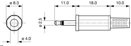
Cable diameter max. 4.0 mm
