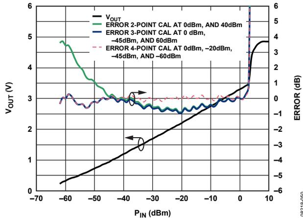
Figure 50. 2.14 GHz Transfer Function, Using Various Calibration Techniques
