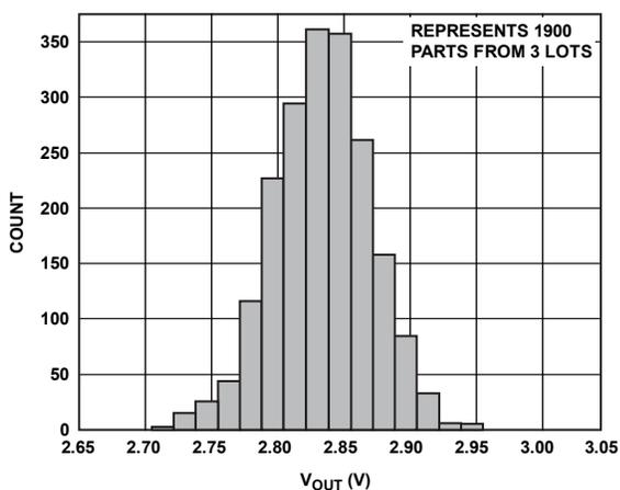
Figure 17. Distribution of  $V_{OUT}$ ,  $P_{IN} = -10$  dBm, 900 MHz
