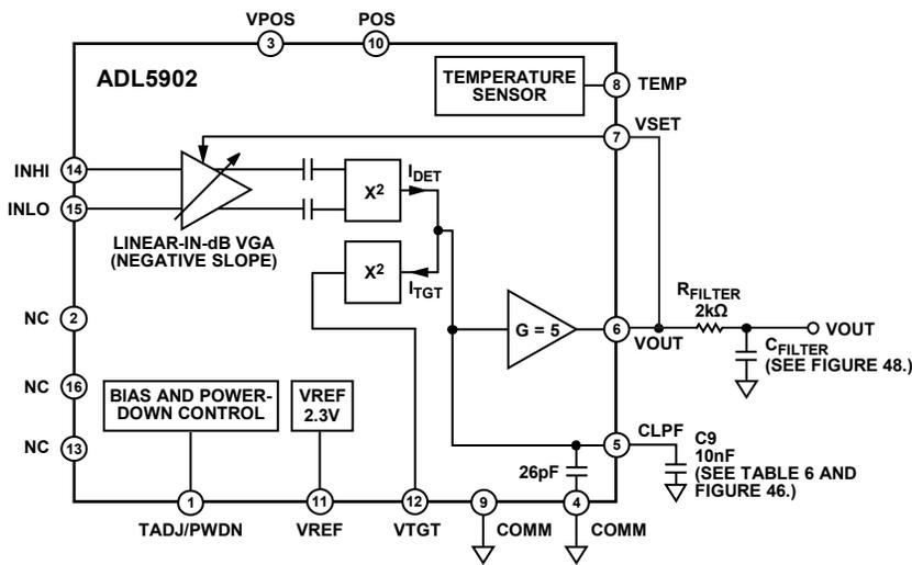
Figure 47. Optimizing Setting Time and Residual Ripple
