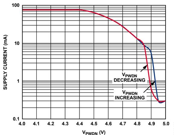
Figure 32. Supply Current vs.  $V_{PWN}$
