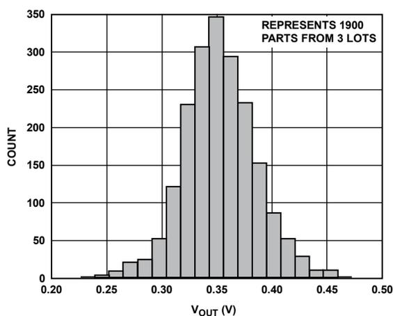
Figure 20. Distribution of  $V_{OUT}$ ,  $P_{IN} = -60$  dBm, 900 MHz
