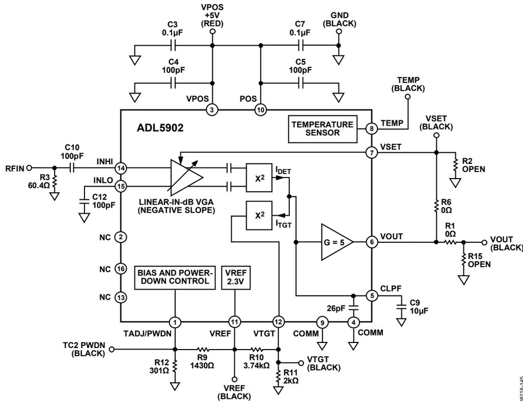
Figure 45. Basic Connections for Operation in Measurement Mode
