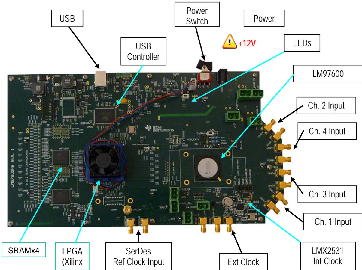
Figure 1: LM97600RB Board Layout
