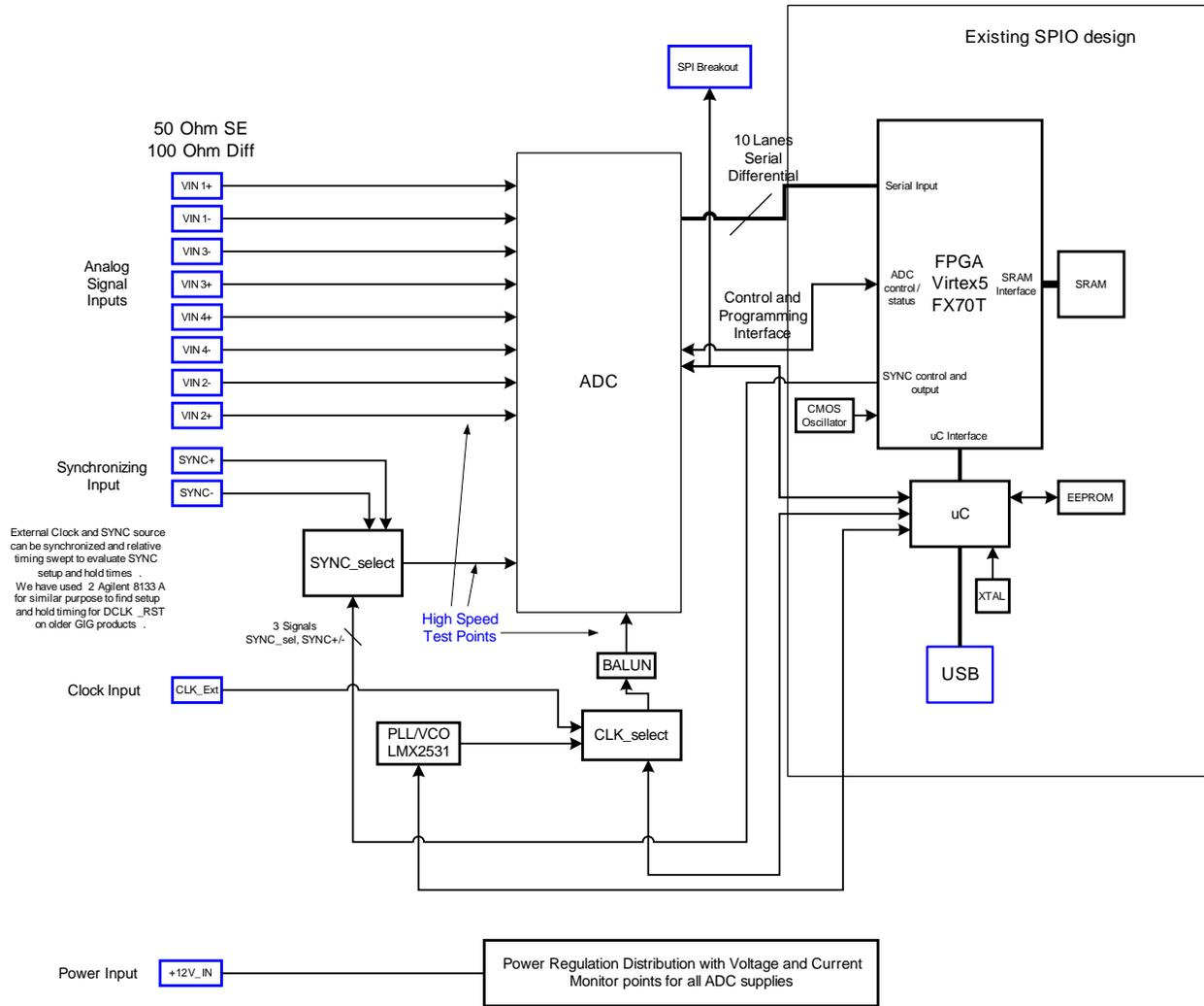
Figure 17: LM97600RB System Block Diagram
