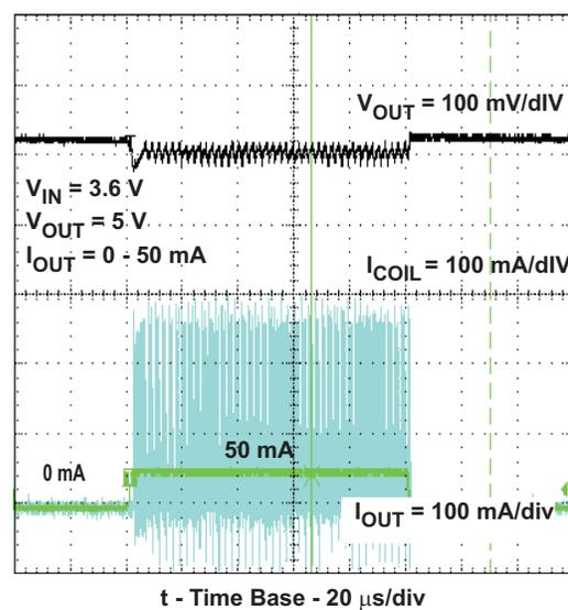
Figure 10. Load Transient Response 0mA–50mA and 50mA–0mA
