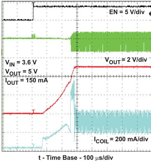
**Figure 15. Startup After Enable – With Load**
