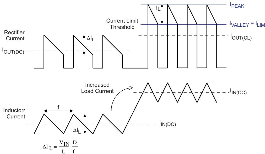
Figure 17. Inductor/Rectifier Currents in Current Limit Operation
