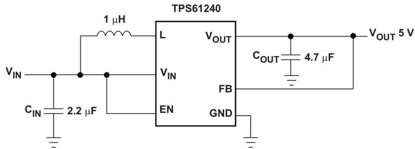
Figure 18. TPS61240-Q1 Fixed 5.0V for HDMI / USB-OTG Applications
