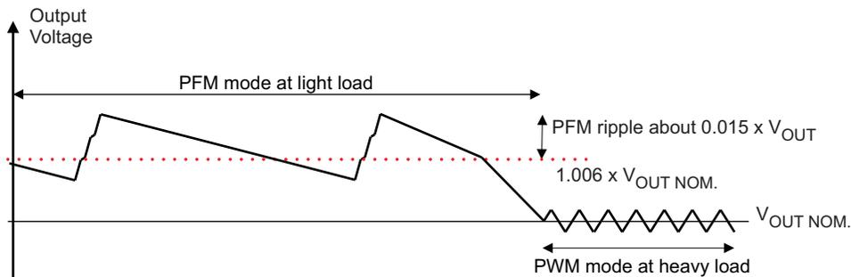
The PFM mode is left and PWM mode entered in case the output current can not longer be supported in PFM mode.
