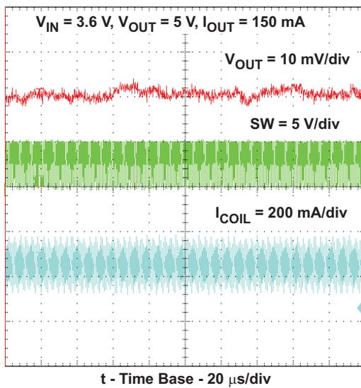
Figure 9. Output Voltage Ripple – PWM Mode
