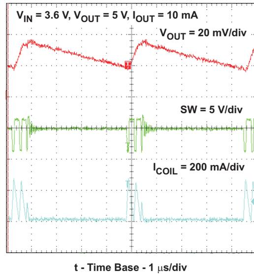
Figure 8. Output Voltage Ripple – PFM Mode
