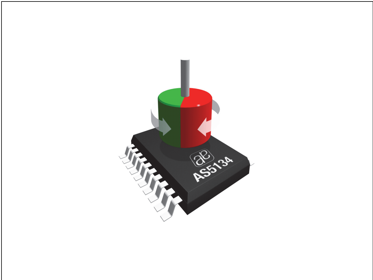
Figure 3. Typical Arrangement of AS5134 and Magnet
