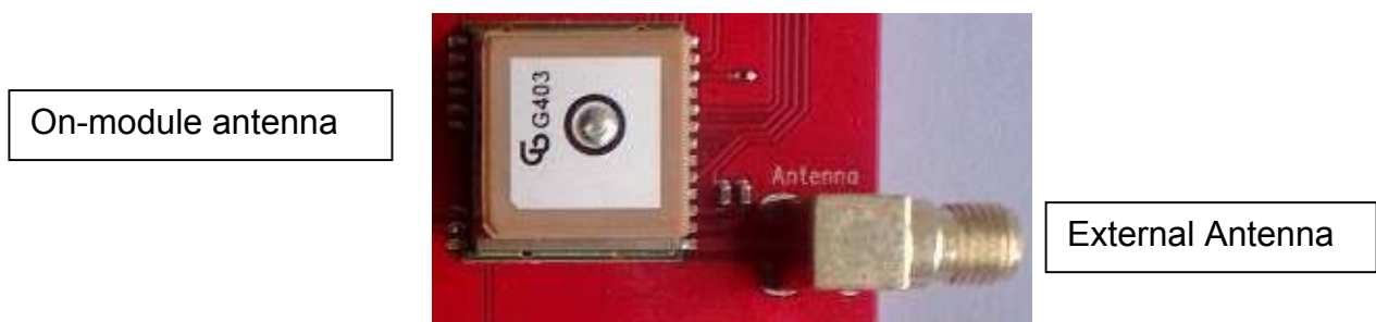
Figure 6: On-module antenna and External Antenna Connector
