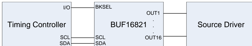
Figure 20. Gamma Control Block Diagram
