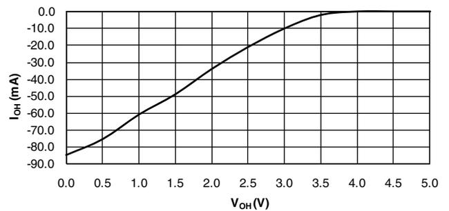
**ATMEL ATF22V10C/CQ OUTPUT SOURCE CURRENT VS. SUPPLY VOLTAGE ( $V_{OH} = 2.4V$ )**
