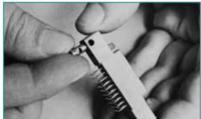
LOCKING BUSHING ACCESSORY INSERTED INTO PC CONNECTOR BODY
