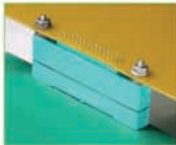
MB to I/O-P Mating Parallel Boards
