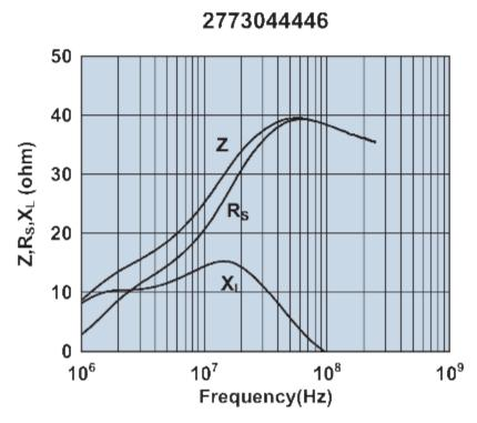
Impedance, reactance, and resistance vs. frequency.
