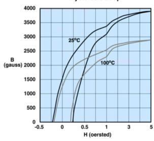
Measured on a 17/10/6mm toroid at 10kHz.
