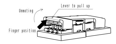
2. After releasing either side, hook the lever on the other side with a finger and lift up to the upper direction, too.
