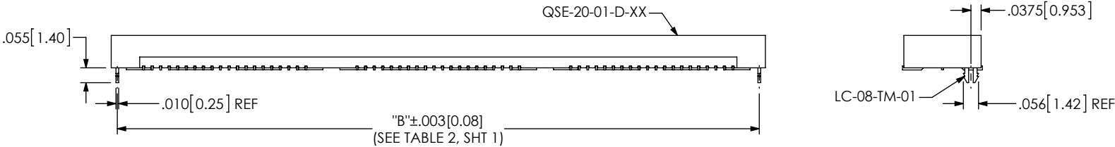
FIG 2 -LC: LOCKING CLIP OPTION (QSE-060-01-XXX-D-LC SHOWN) (DIFFERENT AS SHOWN, OTHERWISE SAME AS FIG 1)
